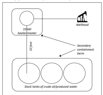
Figure 2-3: Aggregation of equipment at an oil production facility.
