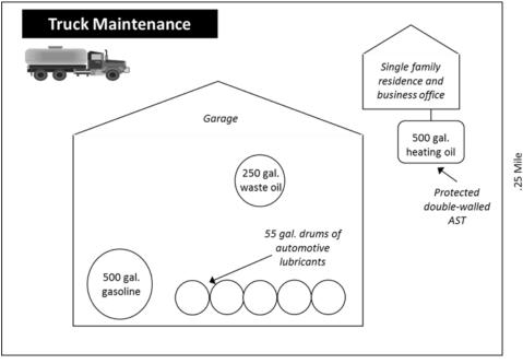
Separation of functions at a dual-purpose facility. Figure 2-6:
