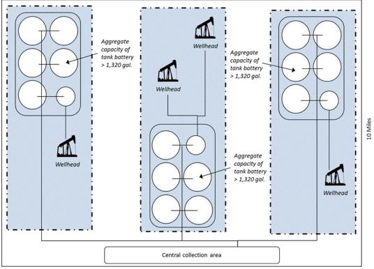
Figure 2-2: Separation of parcels at an oil production facility.
