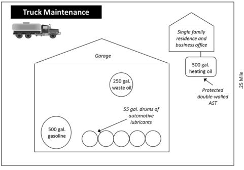
Figure 2-6: Separation of functions at a dual-purpose facility.
