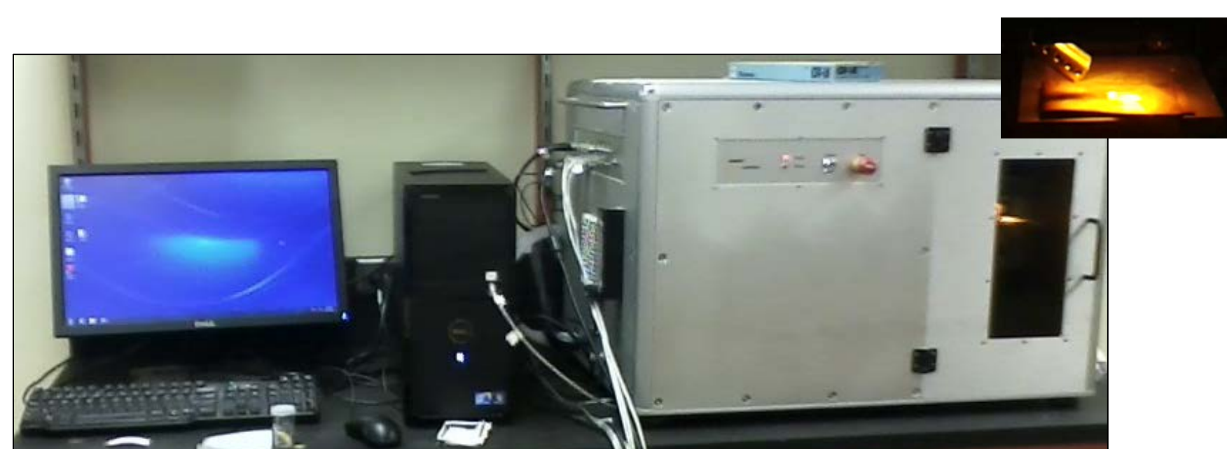
LIBS system (Photon-Machines, Inc.) with insert showing sample stage. Our system is equipped with a pulsed, Q-switched Nd:YAG laser (1064 nm, 10-500 mJ) and a broadband diode array spectrometer.
