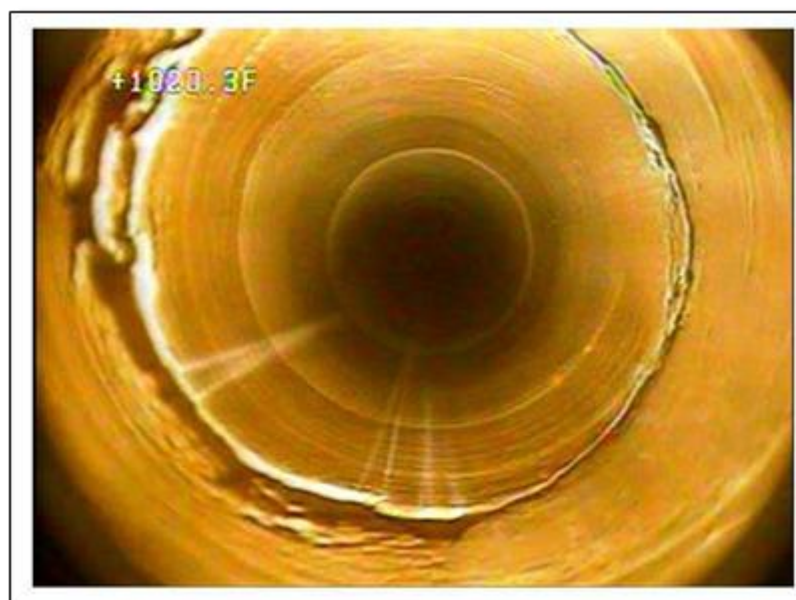
Figure 6. Video still image of saline-water inflow from a bedding-parallel fracture penetrated at 1,026 feet below land surface by the Gleason corehole, western Bradford County, Pennsylvania
