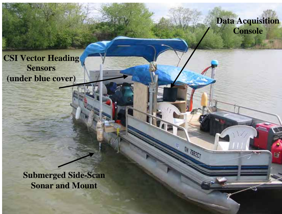
Figure 2-4. Side Scan Sonar System Setup for the Ashtabula River Study
