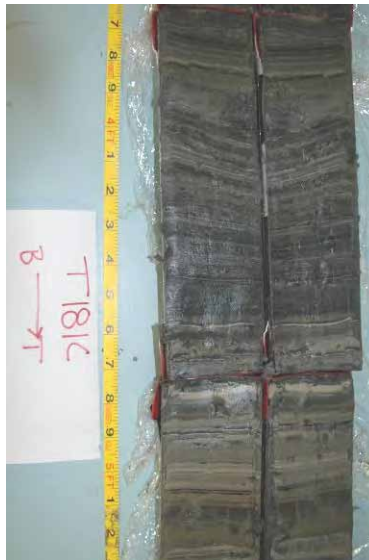
Figure 3-1. Typical Pre-Dredge Sediment Core
