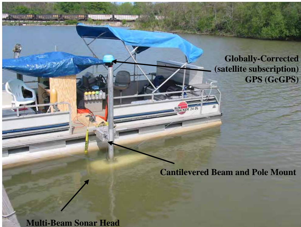
Figure 2-3. Multi-Beam Sonar System Setup for the Ashtabula River Study
