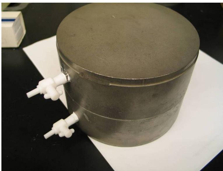
Fig. 1. A picture of the testing apparatus showing the two halves of the permeability cell placed together, and showing placement of the valves. Not shown - valves are also placed on opposite sides of each half.
