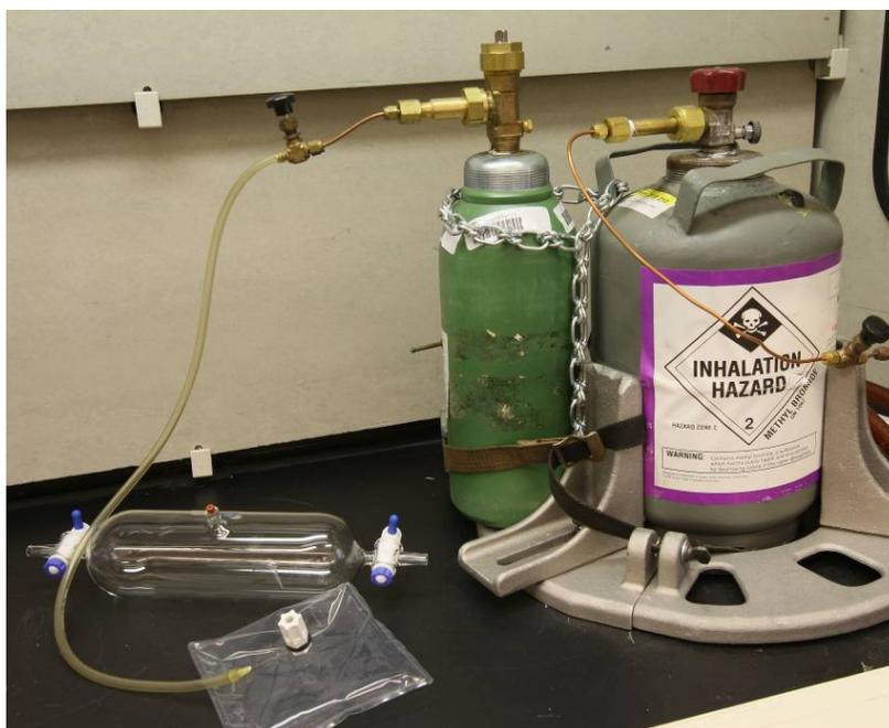
Fig. 2. A picture showing the transfer line (including the fumigant tank, copper tubing, valve, Tygon tubing, and syringe needle). A Tedlar bag and a 1 L glass mixing chamber are also shown in the picture.
