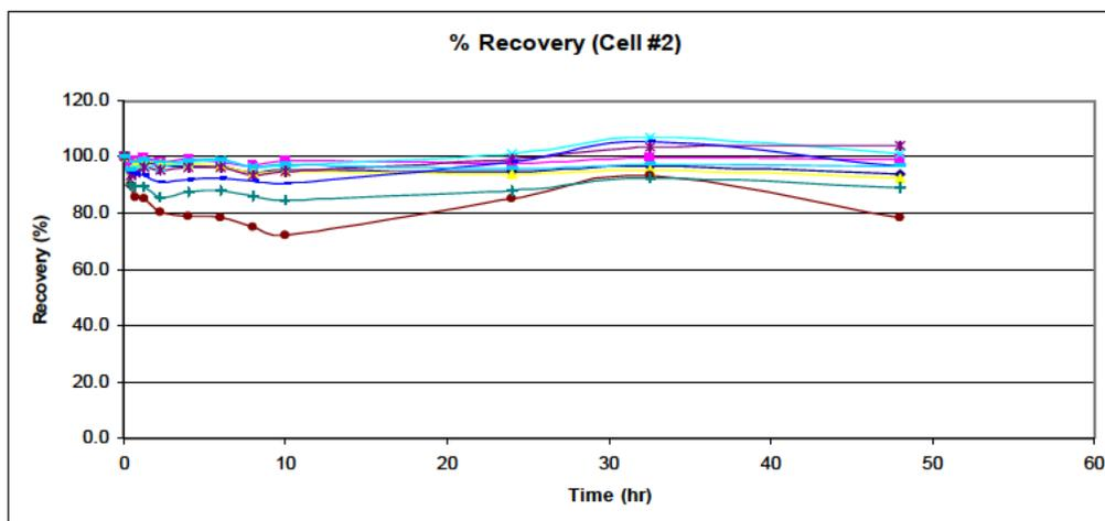
Fig 3. An example of the recoveries of various fumigants from the permeability cell monitored over time. The recoveries represent total amount present in both chambers relative to the amount present at the initial 5 min sampling.
