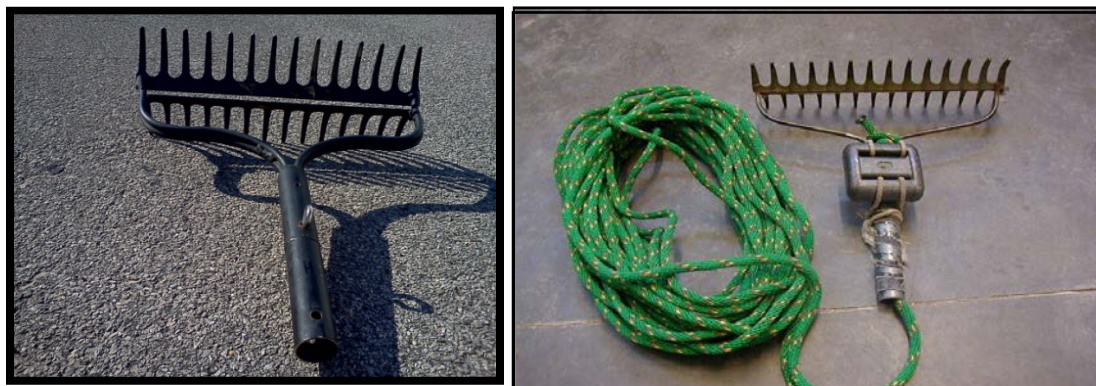
Figure 6.2 Examples of rake sampler used for macrophyte assemblage characterization.
