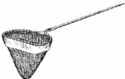
Figure 6.9 D-frame net (500 \mu\text{m} mesh) used for collecting benthic macroinvertebrates.
