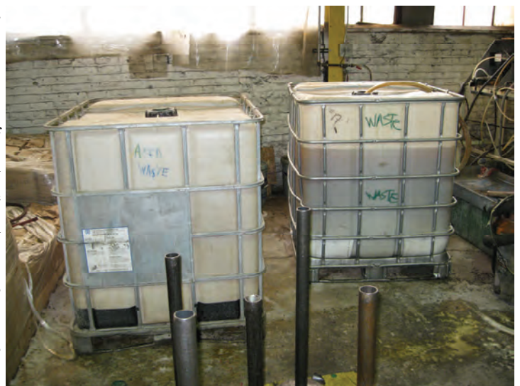
Plastic totes that were filled with Superfinish etch waste which, once full, were taken out to a storm drain in the facilities courtyard and drained to the combined sanitary sewer.
