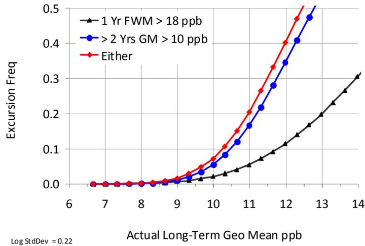
X Axis: LTFWM of STA discharge. An STA operating with a LTGM < 10 ppb would be in compliance with the phosphorus criterion. Y-Axis: Predicted excursion frequencies for each component of the two-part test. The red line depicts the probability that either of the tests will be exceeded in any year.
