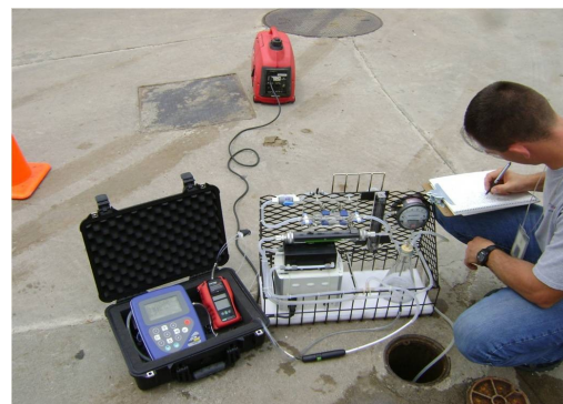
Sampling methane from a groundwater monitoring well at a LUST site
