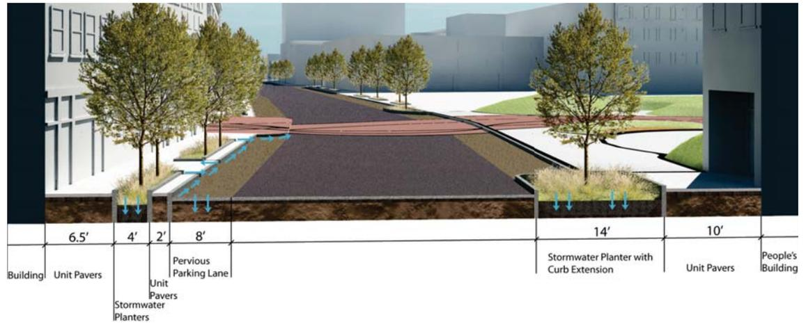
Figure 45. Stormwater infiltration planters along Summers Street.
