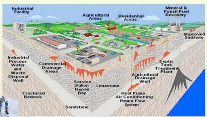
**UIC Program** - regulating the disposal of fluids into the subsurface from simple devices (floor drains) to complex system (injection wells).
