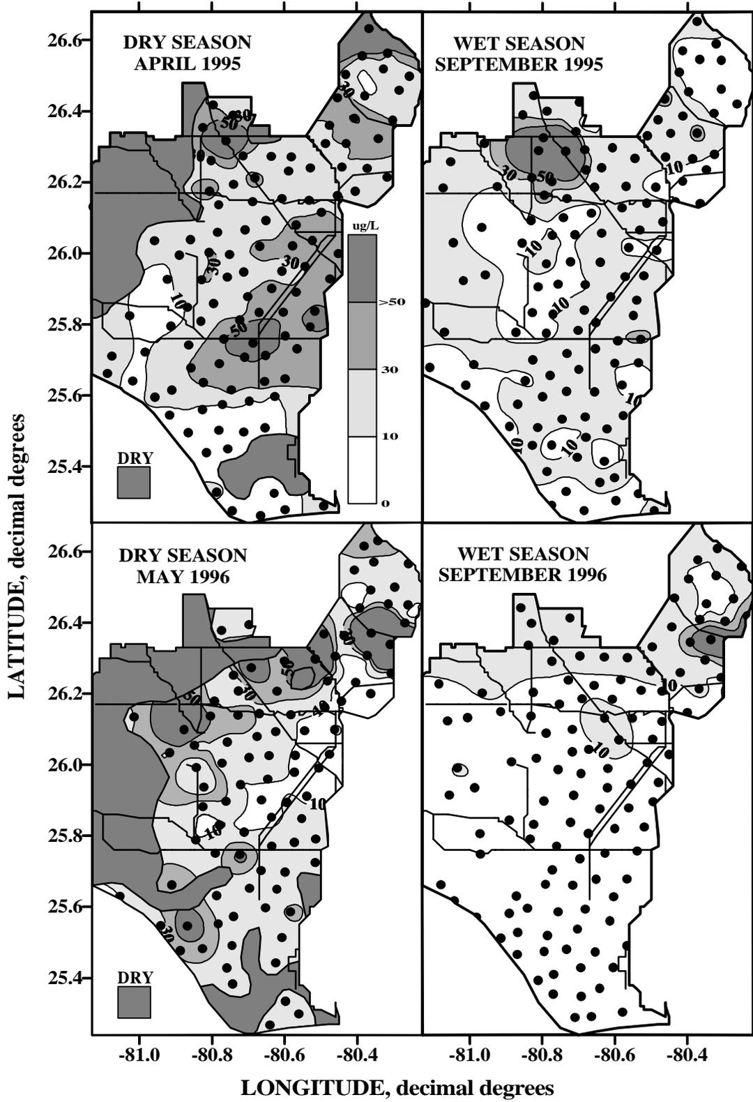
Figure 8.49 Kriged surfaces showing TP in the marsh for each sampling cycle based on sampling data.
