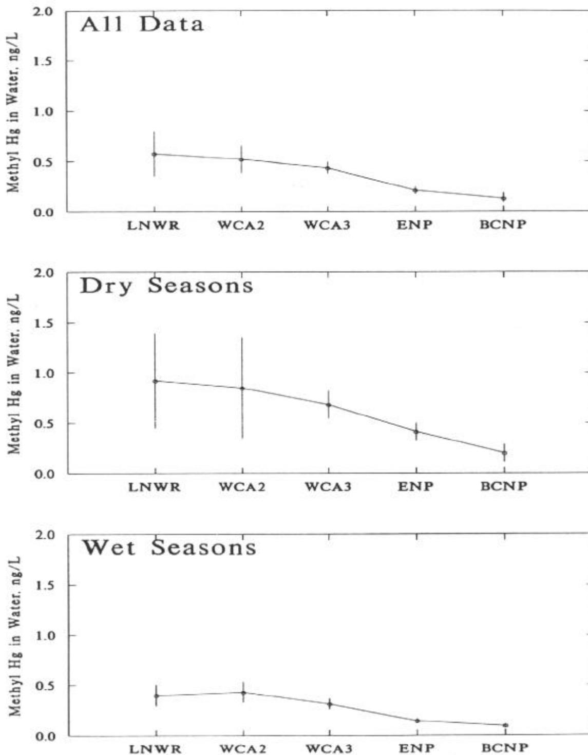
Figure 8.36 Median values of marsh MeHg for subareas with vertical lines indicating the 95% confidence interval for each median.
