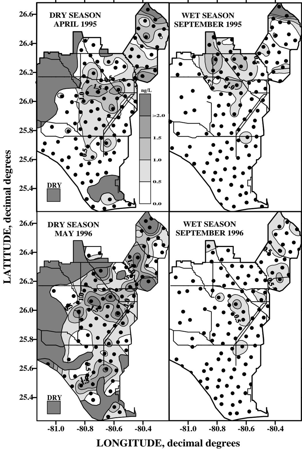
Figure 8.50 Kriged surfaces indicating marsh MeHg concentrations during each of the sampling cycles.
