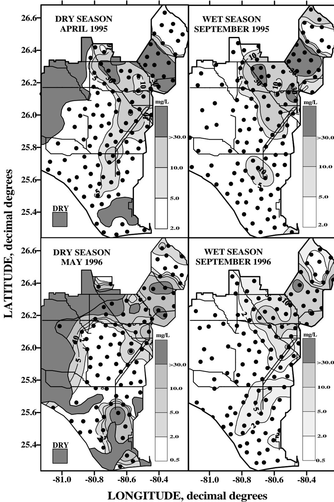
Figure 8.48 Kriged surfaces indicating marsh  $\text{TSO}_4$  concentrations during each sampling cycle.
