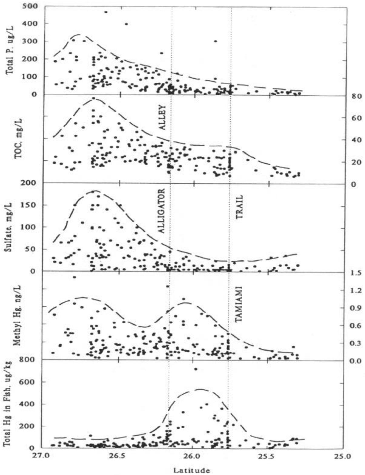
Figure 8.13 Plot of selected constituents showing latitudinal gradients in canals.
