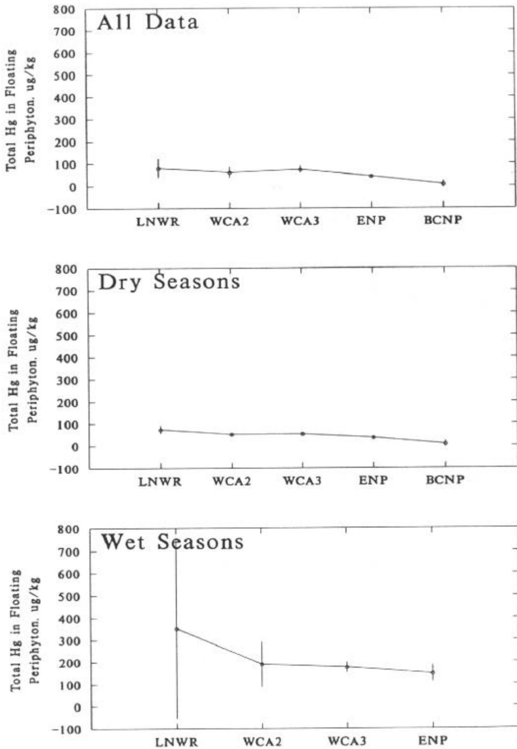
Figure 8.40 Median values of THg in floating periphyton for subareas with a vertical line indicating the 95% confidence interval for each median.
