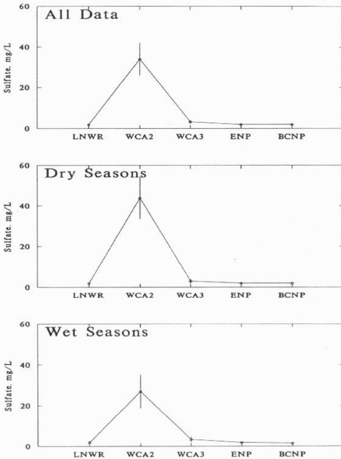
Figure 8.29 Median marsh  $\text{TSO}_4$  values for subareas with a vertical line indicating the 95% confidence interval for each median.
