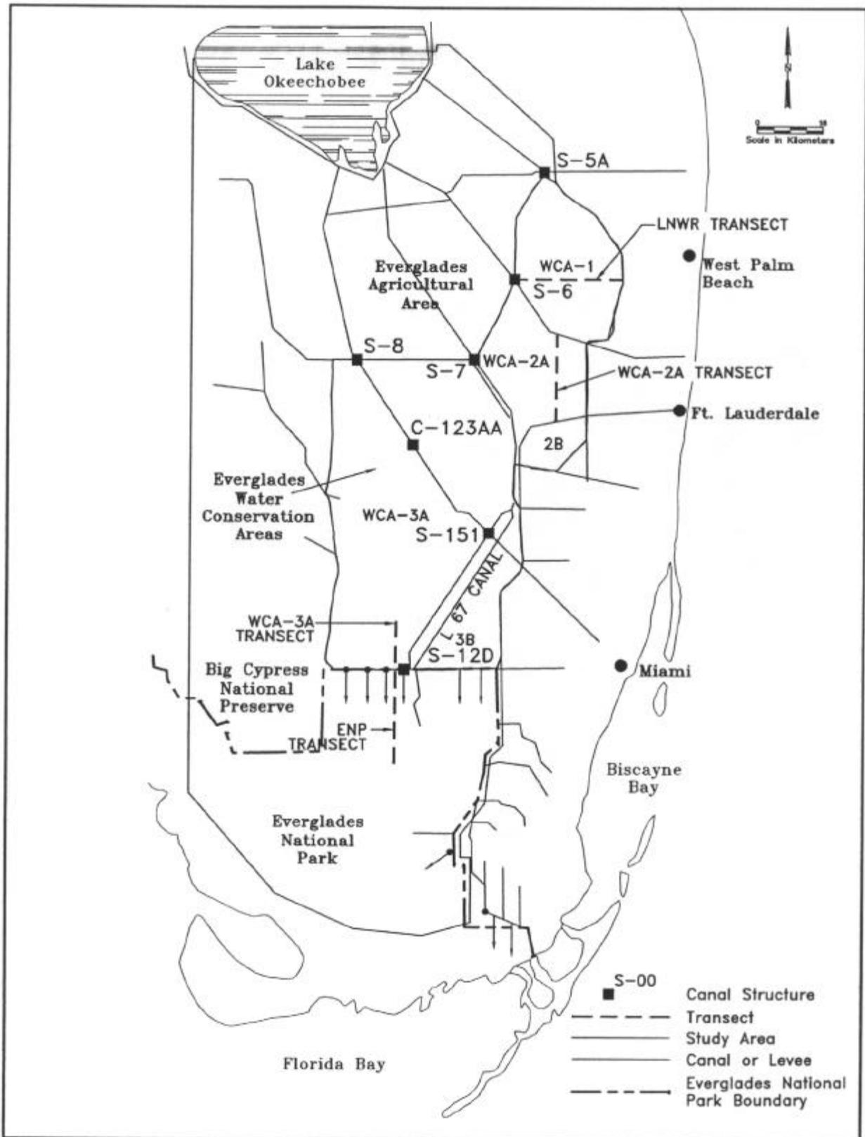
Figure 8.14 Location of four marsh transects sampled in April 1994 and canal water control structures sampled on a biweekly basis from February 1994 through February 1997.
