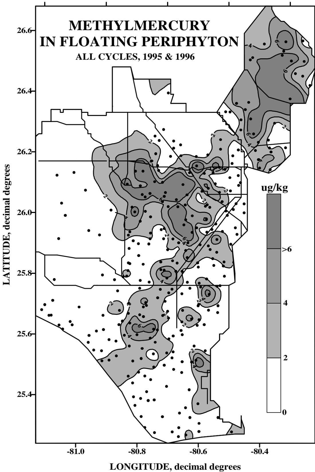
Figure 8.51 Locations of floating periphyton samples with kriged surfaces indicating concentrations of MeHg in floating periphyton.
