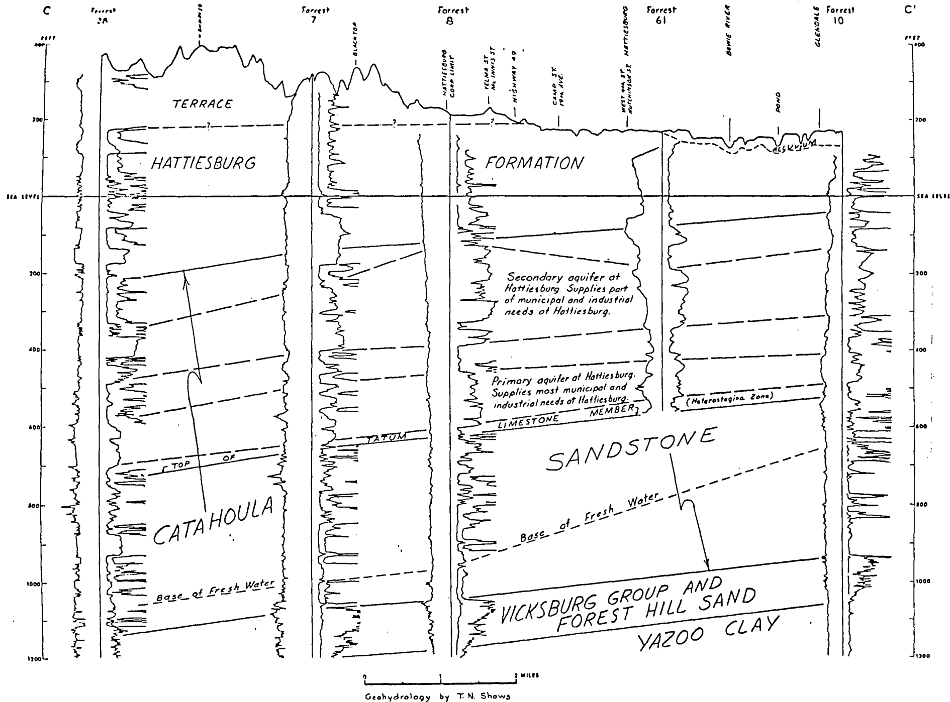
Fig. 1. Geohydrologic section (C-C') through the Hattiesburg area
