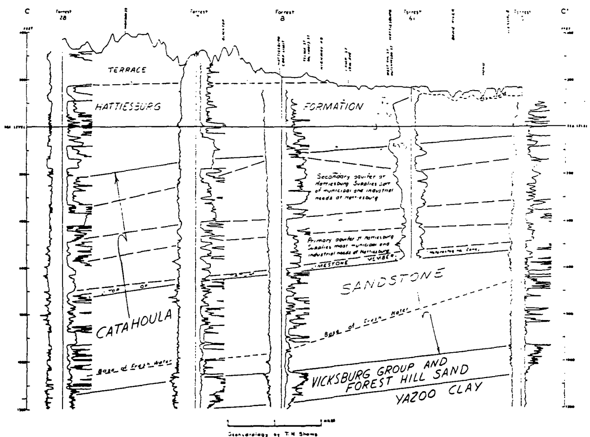
Fig. 22. Geohydrologic section (C-C') through the Hattiesburg area
