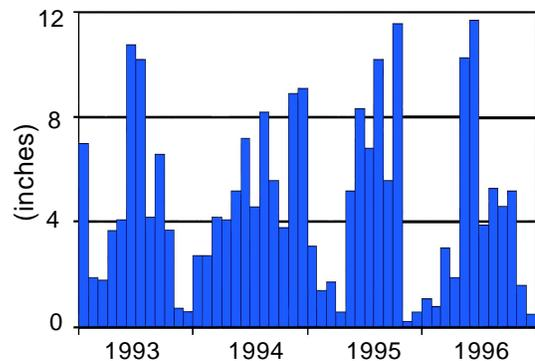
**FIGURE 20.** Monthly rainfall (inches) from 1993 to 1996 at S-8, a pumping station that provides flood control for part of the EAA by discharging into the Everglades.
