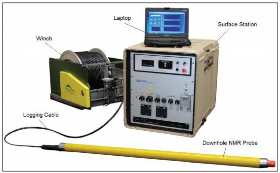
Exhibit V-25: Small-Diameter NMR Probe And System Components
