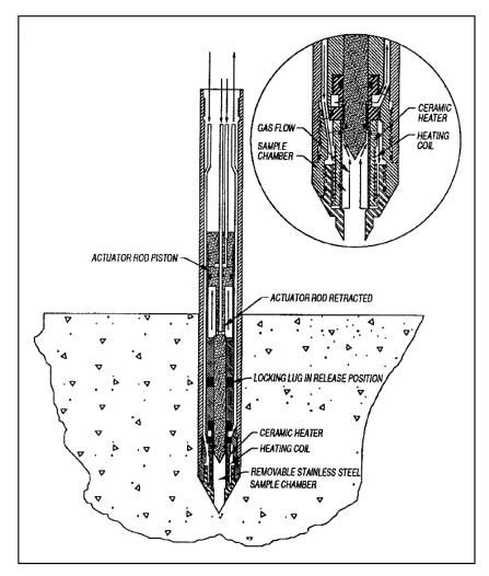
Exhibit V-36: Schematic Of TDS Probe In Ready-To-Sample Position
