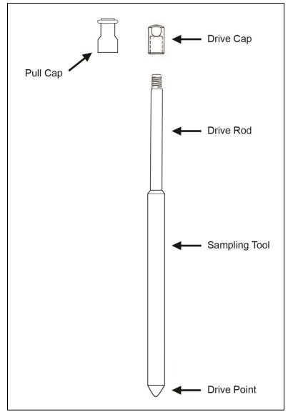
Exhibit V-6: Schematic Drawing Of A Single-Rod Direct Push System
