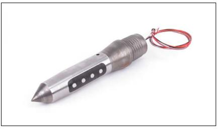
Exhibit V-24: Small-Diameter Direct Push EC Probe
