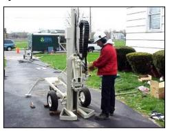
b) Percussion hammer system mounted on a track rig
