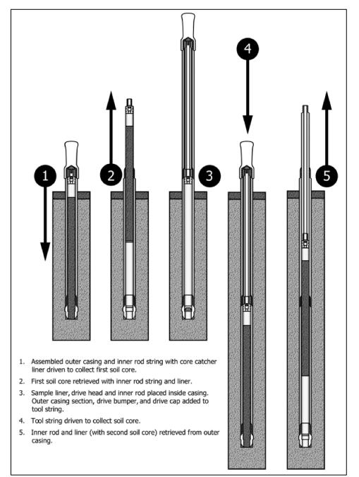
Exhibit V-10: Dual-Tube Soil Sampler Operation
