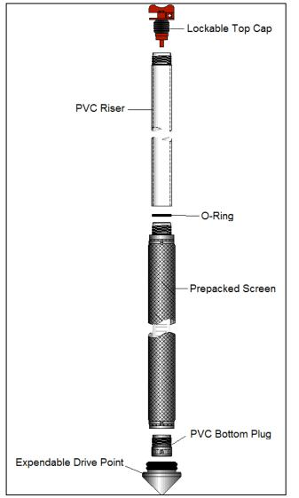
Exhibit V-16: DP-Installed Prepack Screen Monitoring Well
