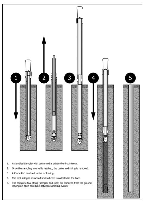
Exhibit V-9: Piston Soil Sampler Operation
