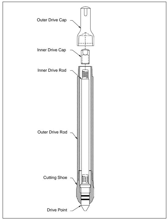
Exhibit V-7: Schematic Drawing Of A Dual-Tube Direct Push System
