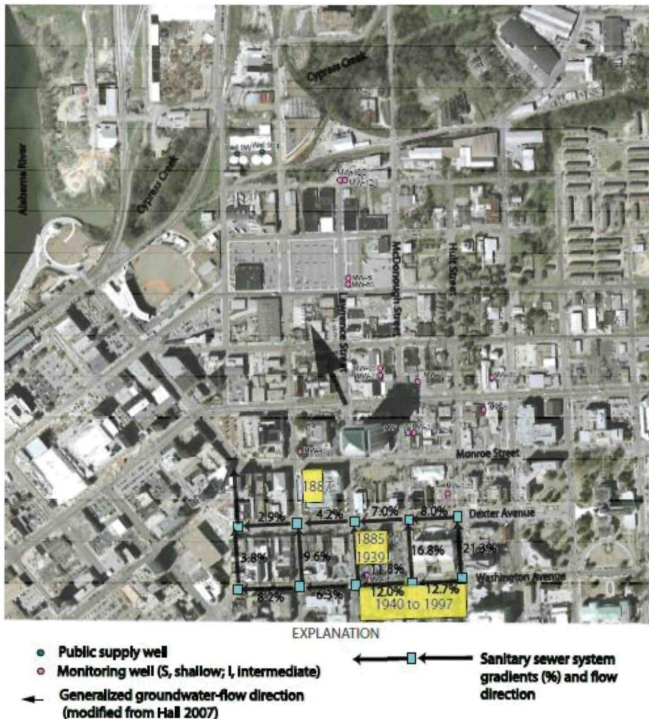
Figure 17. Location of sanitary sewer system, slopes from outfalls, and flow direction.
