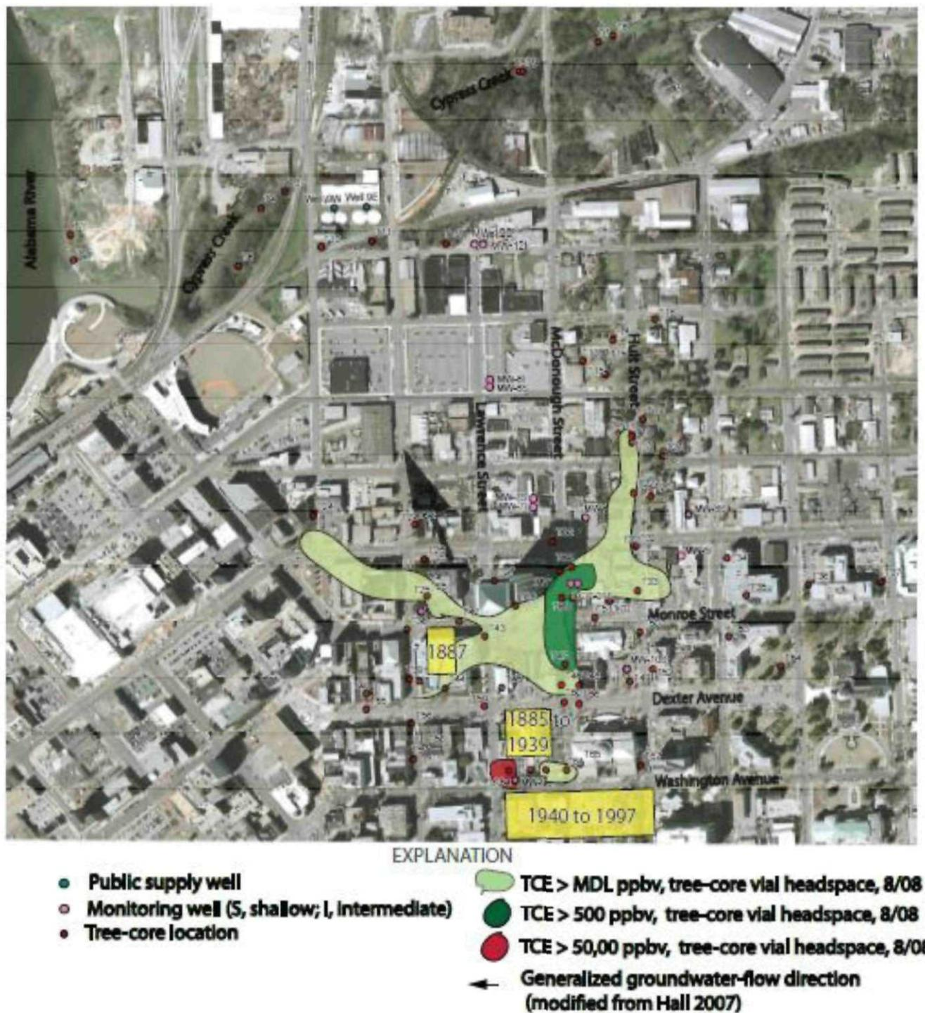
Figure 14b. Locations of TCE in tree-core vial headspace, ppbv, data from USGS sampling August 2008, with former locations and dates occupied by a major commercial printing industry.
