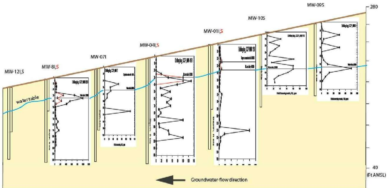
Figure 11. Cross section showing PID results for wells installed in 2000 during the USEPA RI (data from Black & Veatch 2002; data interpretation by USGS).
