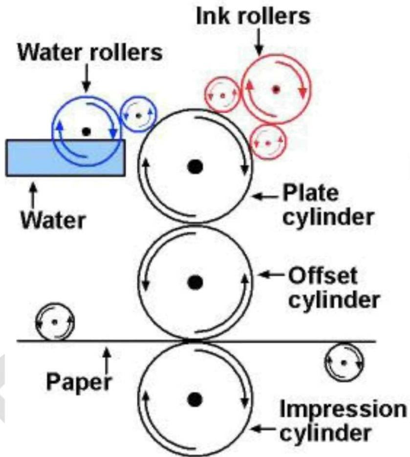
Figure 25. Offset printing process that uses blanket wash on the offset, or blanket, cylinder.
