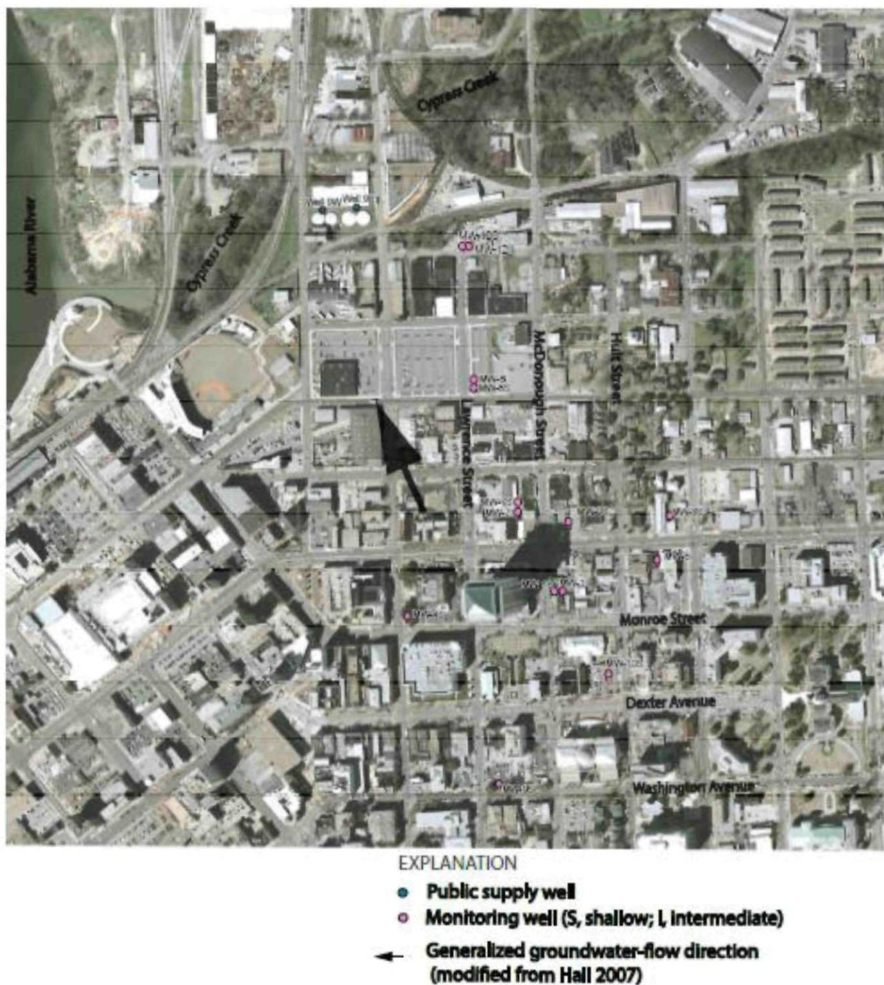
Figure 3. Location of public supply and shallow (S) and intermediate (I) monitoring wells and generalized groundwater-flow direction at the Capital City Plume (CCP) Site, July 2007, Montgomery, Alabama (modified from Hall 2007).
