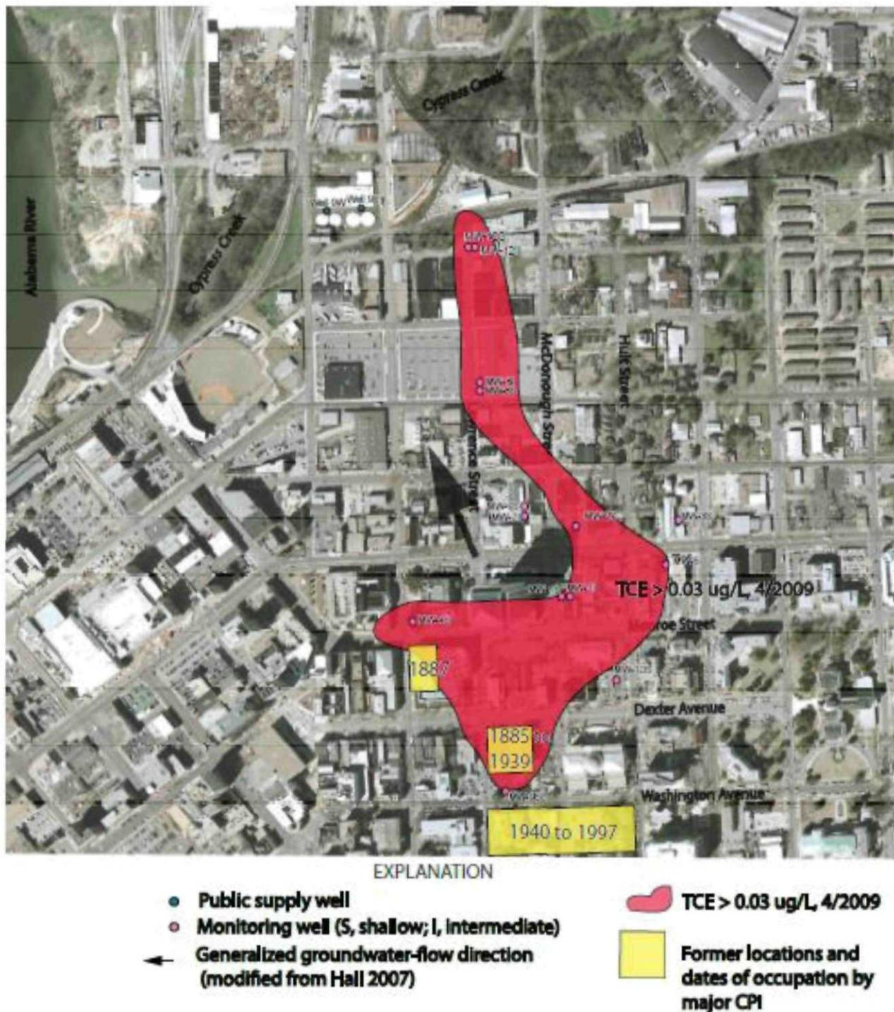
Figure 13b. Locations of TCE in groundwater, data from USGS sampling April--May 2009, with former locations and dates occupied by a major commercial printing industry. TCE data for 9W from MWWSSB.
