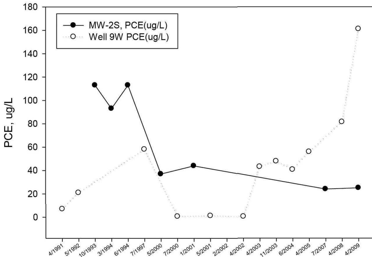
Figure 22a. Trends for PCE in MW-2S and 9W over time. PCE has decreased in MW-2S since 1993, and a roughly equal increase of PCE has been observed in downgradient and nonpumping well 9W.
