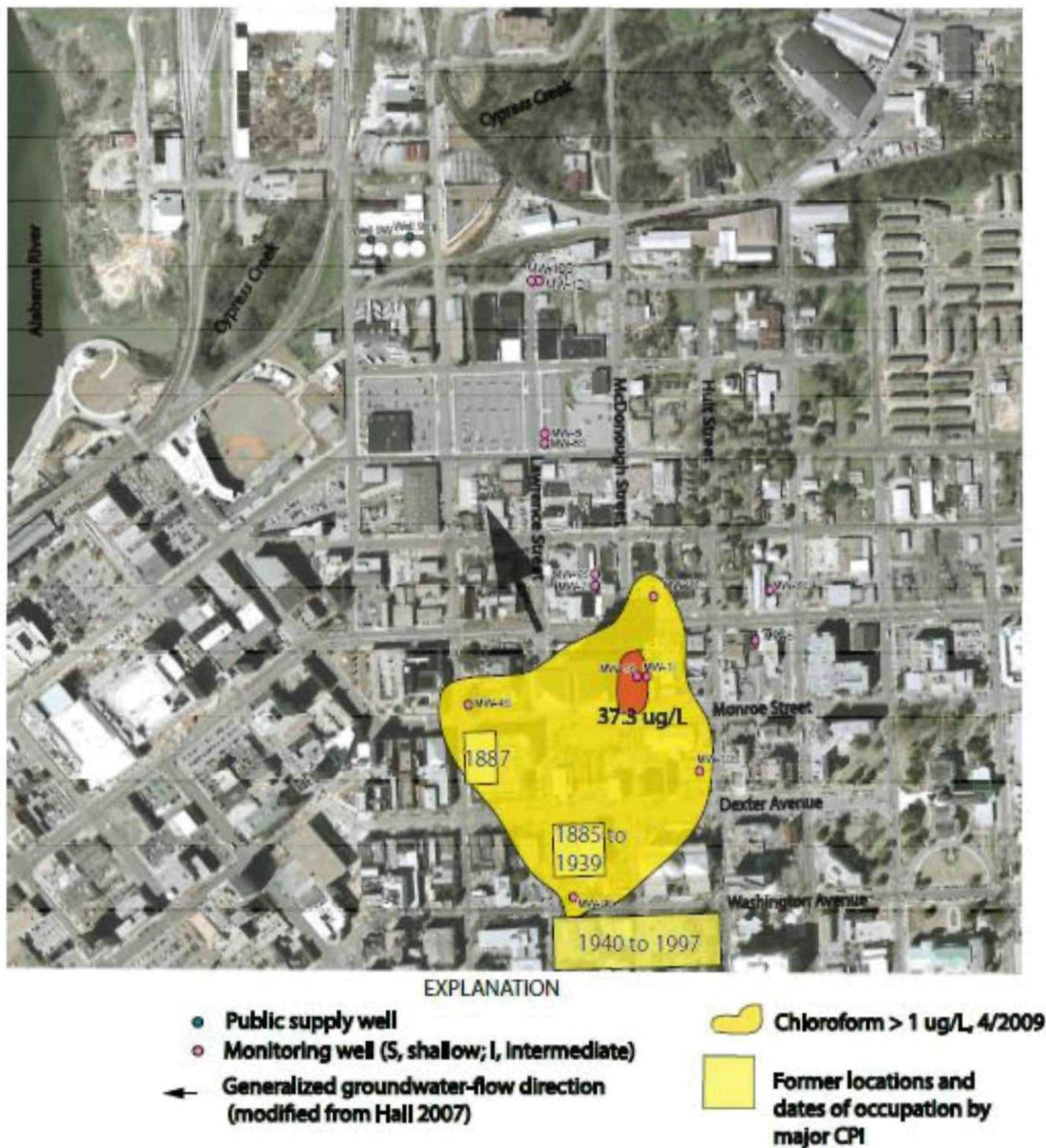
Figure 16. Monitoring wells with chloroform plume April–May 2009.
