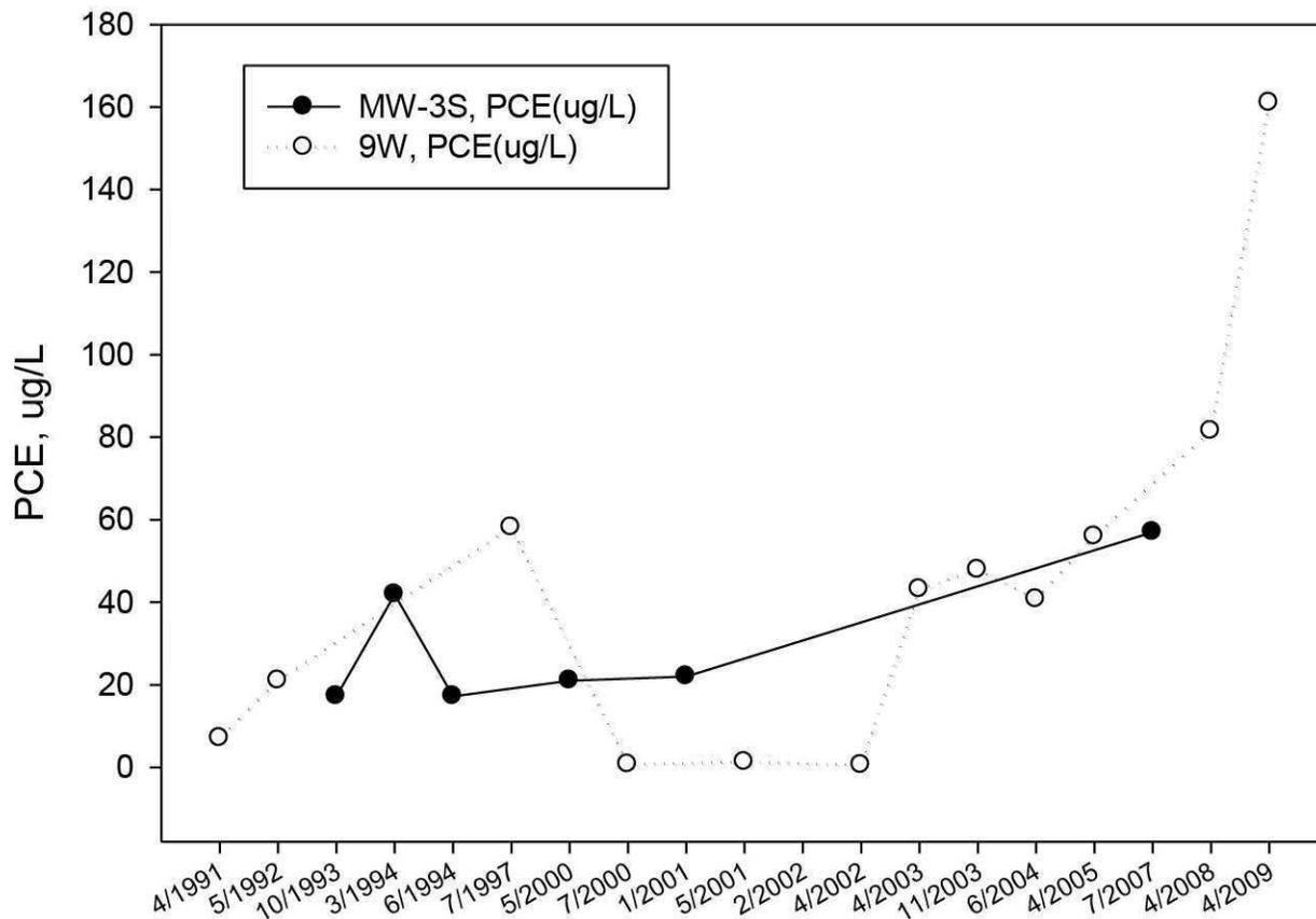
Figure 22b. Trends for PCE in MW-3S and 9W over time. PCE in 9W decreased as PCE in well MW-3S slightly increased. Since 2003, PCE has increased in both wells, although to a greater extent in 9W.
