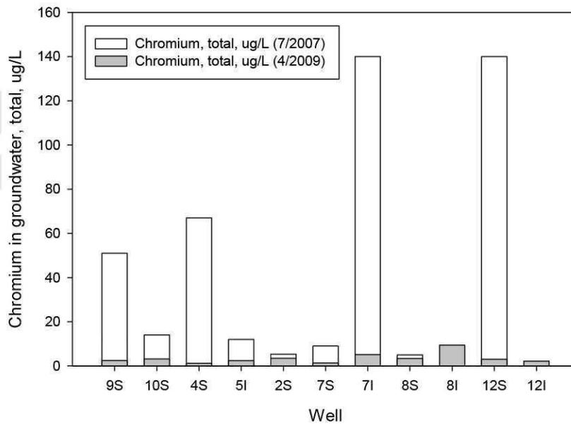
Figure 15. Comparison of groundwater sample (a) turbidity and (b) total chromium for sampling events on July 2007 and April–May 2009.
