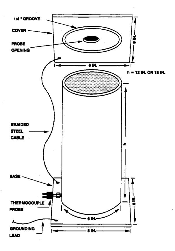
FIG 1. Test Container and Cover
