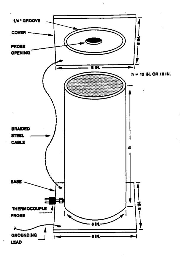
FIG 1. Test Container and Cover
