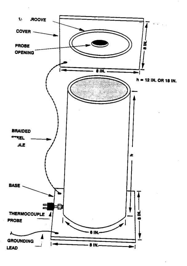
FIG 1. Test Container and Cover
