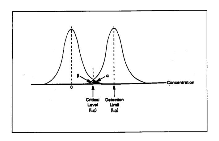
FIG. 1. Graphical Representation of Detection Limit and Critical Level
