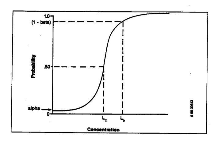
FIG. 2. Probability of Detection Versus Concentration
