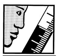
USE GOOD STICKING PRACTICES: Slowly lower the gauge stick, let the stick gently touch bottom, and quickly bring it back up. Read the depth of the fuel indicated by the wet mark on the stick to the nearest 1/8 inch.
