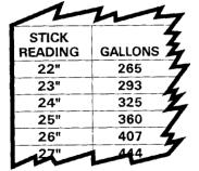
The easiest way to explain this procedure is with an example. Let's say you have a stick reading of 23-3/8 inches and you need to figure how many gallons are in your tank.
