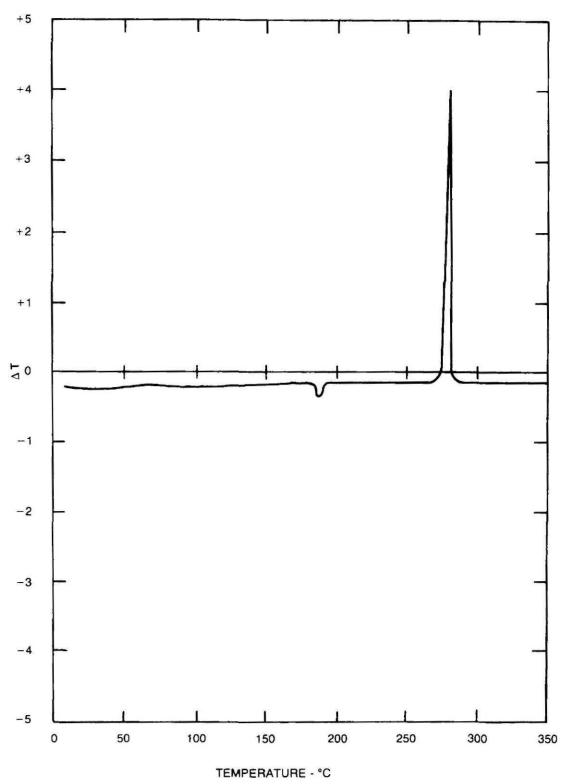
Figure 8-92. DTA curve for PBXN-5.
