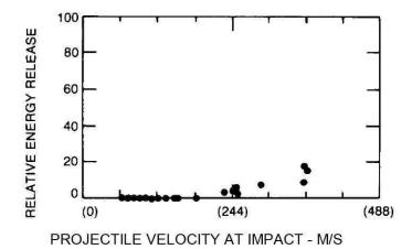
Figure 8-67. Susan test results for TNT.
