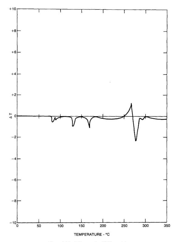
Figure 8-76. DTA curve for 80/20 amatol.
