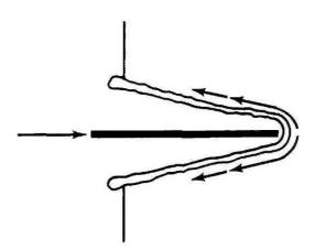
Figure 4-13. Shaped charge penetration.
