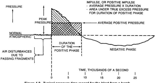
Figure 4-9. Typical pressure-time record for the blast from a bomb.
