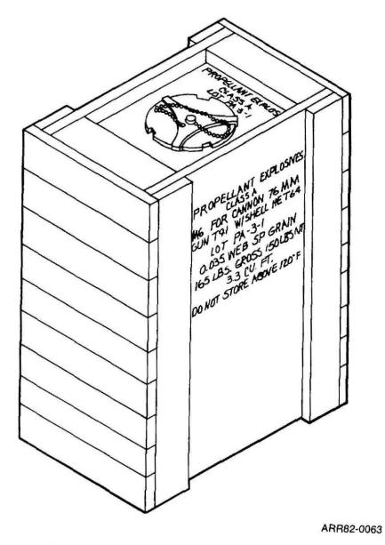
Figure 14-2. Metal lined wood box for packing solid propellants, including markings.
