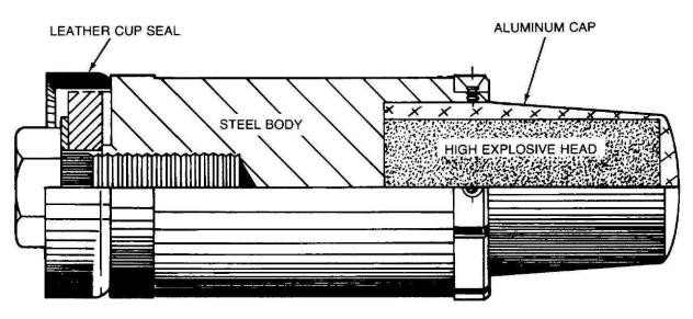
Figure 5-7. Scaled drawing of the SUSAN projectile. The high explosive head is 4 in. long and 2 in. in diameter (102 m x0.051 m).
