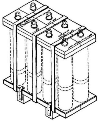
ARR82-0065 Figure 14-4. Palletized large caliber high explosive projectiles, including marking.
