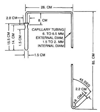
Figure 5-1. Vacuum stability test.
