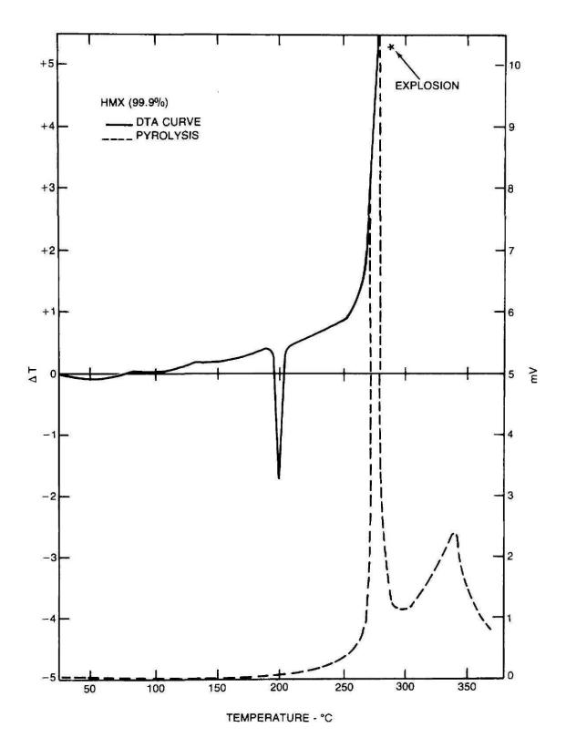
Figure 8-16. DTA curve for HMX.
