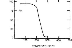
Figure 8-75. TGA curve for ammonium nitrate.
