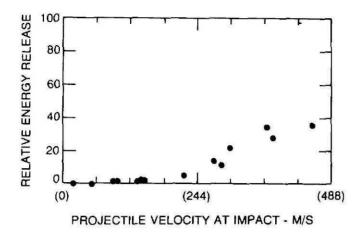
Figure 8-79. Susan test results for composition B3.
