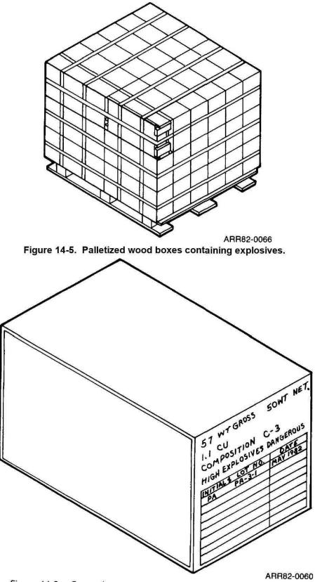
Figure 14-6. Carton for packing high explosives, including marking.
