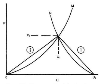
Figure 4-5. Shock properties in the P-u plane.
