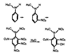
Figure 8-34. Nitration and hydroylsis of methylaniline.
