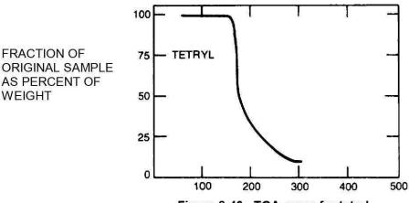
Figure 8-40. TGA curve for tetryl.
