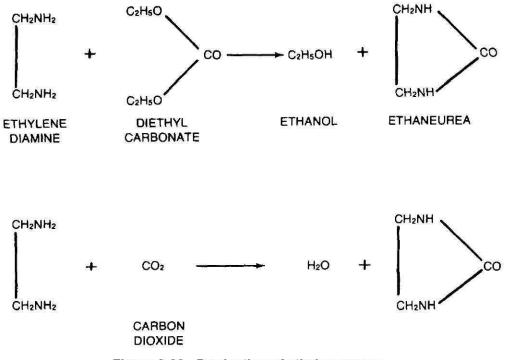
Figure 8-23. Production of ethyleneneurea.
