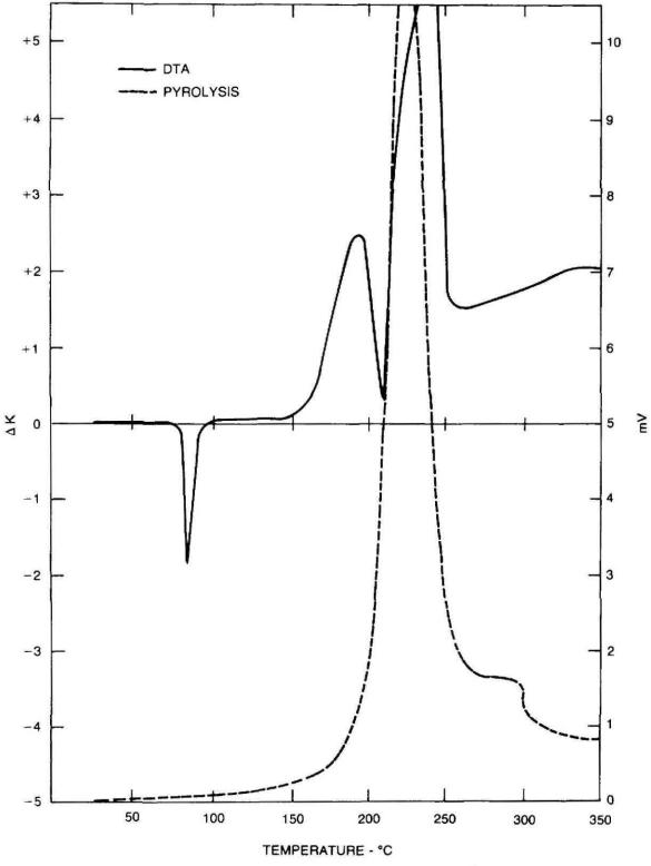
Figure 8-82. DTA curve for 75/25 cyclotol.
