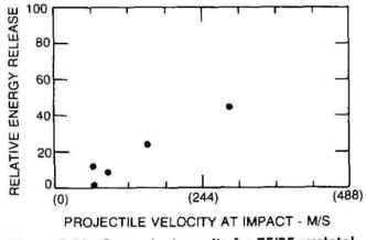
Figure 8-80. Susan test results for 75/25 cyclotol.
