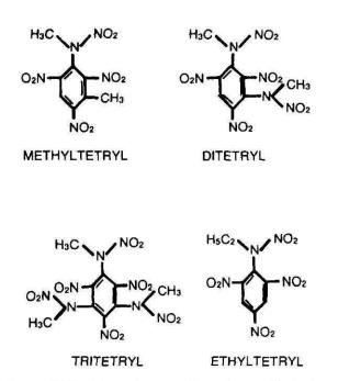
Figure 8-33. Homologs and analogs of tetryl.
