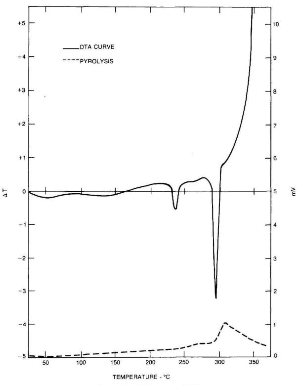
Figure 8-44. DTA curve for DATB.
