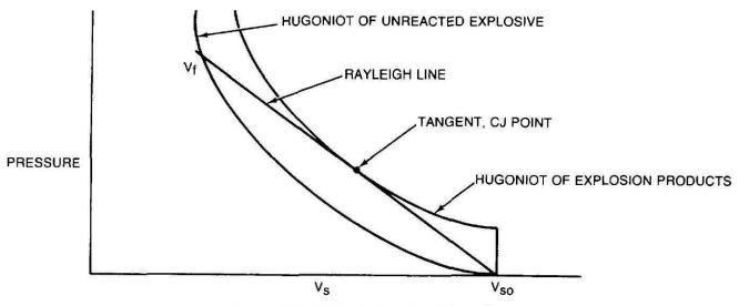
Figure 4-8. P-Vs plot during detonation.
