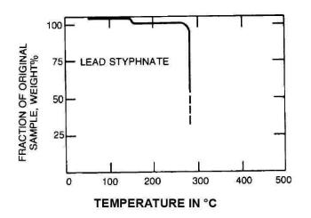
Figure 7-8. TGA curve for lead styphnate.
