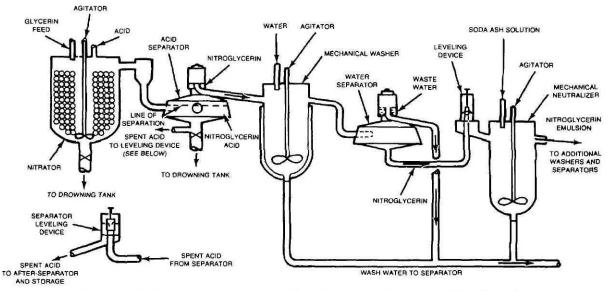
Figure 8-8. Biazzi continuous method for manufacturing nitroglycerin.
