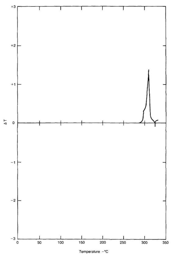
Figure 7-2. DTA curve for lead azide.
