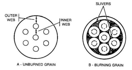
Figure 9-2. Web thickness and direction of burning through a progressively burning grain.
