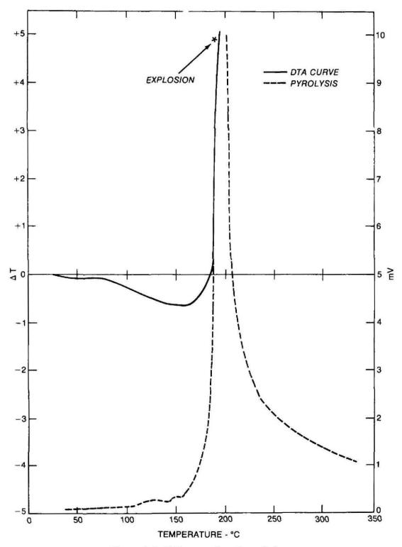
Figure 8-5. DTA curve for nitrocellulose.
