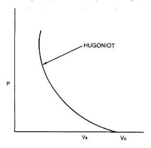
Figure 4-6. Shock properties in the P-Vs plane.
