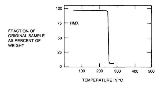
Figure 8-17. TGA curve for HMX.
