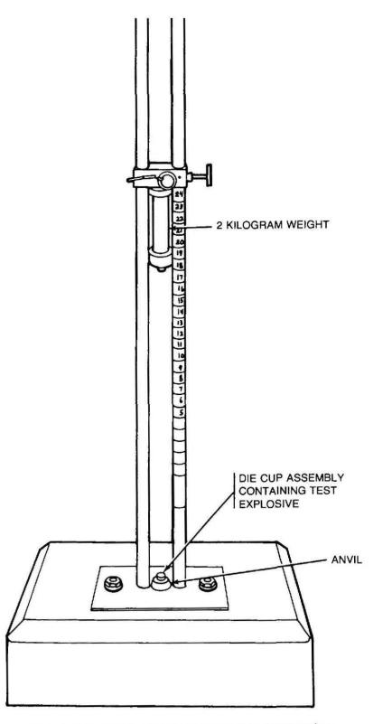
Figure 5-4. Picatinny Arsenal impact test apparatus.
