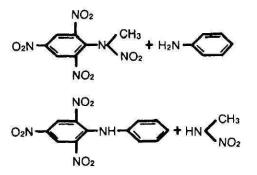
Figure 8-32. Reaction of tetryl with aniline.
