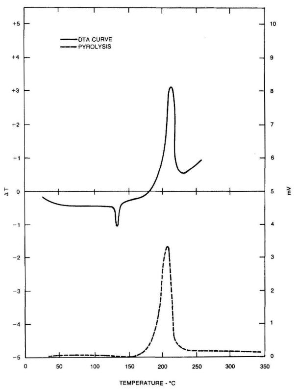
Figure 8-39. DTA curve for tetryl.
