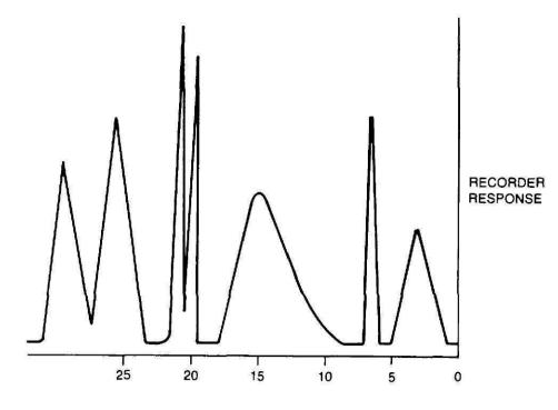
Figure 13-1. Gas chromatograph output.
