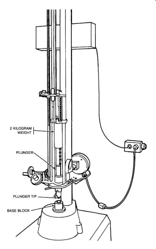
Figure 5-6. Bureau of Mines impact test apparatus.
