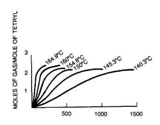
TIME, MINS Figure 8-38. Kinetic gas-evolution curves in the decomposition of tetryl.
