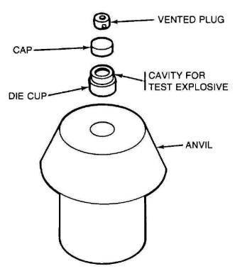
Figure 5-5. Parts of Picatinny Arsenal test apparatus.
