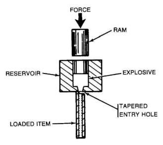
Figure 8-91. Injection loading operation.
