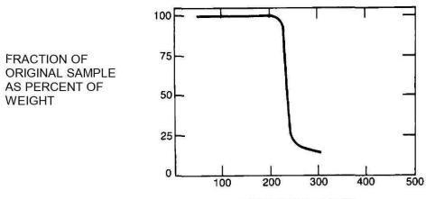
TEMPERATURE IN °C Figure 8-28. TGA curve for nitroguanidine.
