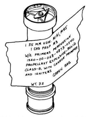
Figure 14-3. Metal containers for propelling charges, including marking.
