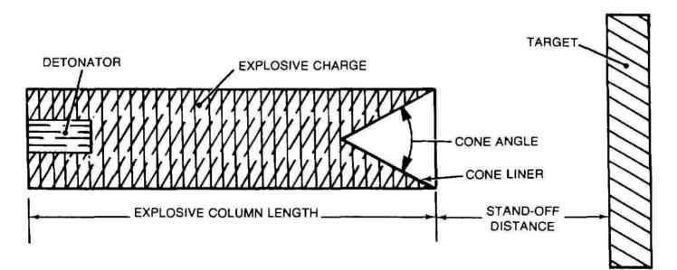
Figure 4-11. Shaped charge and target.
