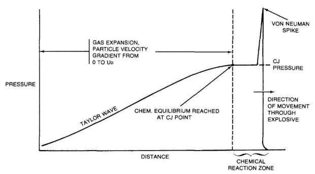
Figure 4-7. Detonation wave.
