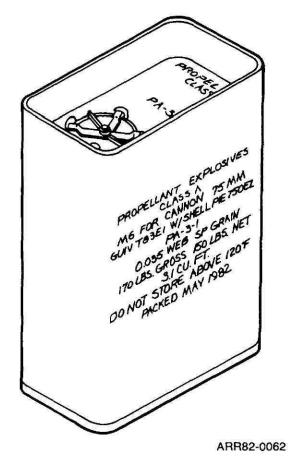
Figure 14-1. Steel box for packing solid propellants, including marking.
