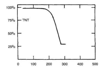
Figure 8-69. TGA curve for TNT.
