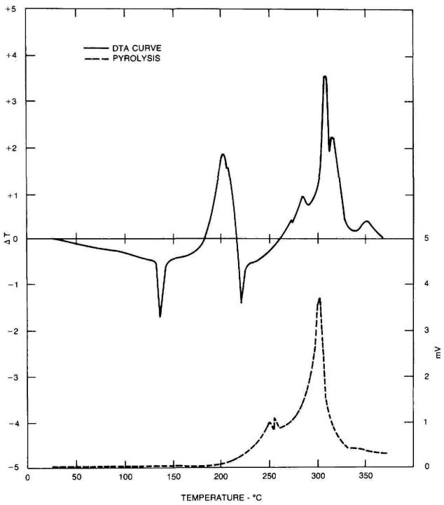
Figure 8-42. DTA curve for ammonium picrate.
