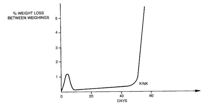
Figure 6-1. 90°C Dutch weight loss test results.
