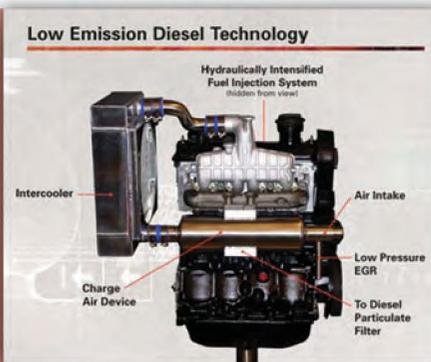
*“The innovative design allows an average fuel economy improvement of 30 to 40 percent over gasoline engines and produces the lowest known engine-out NOx ever achieved by any diesel engine.”*
