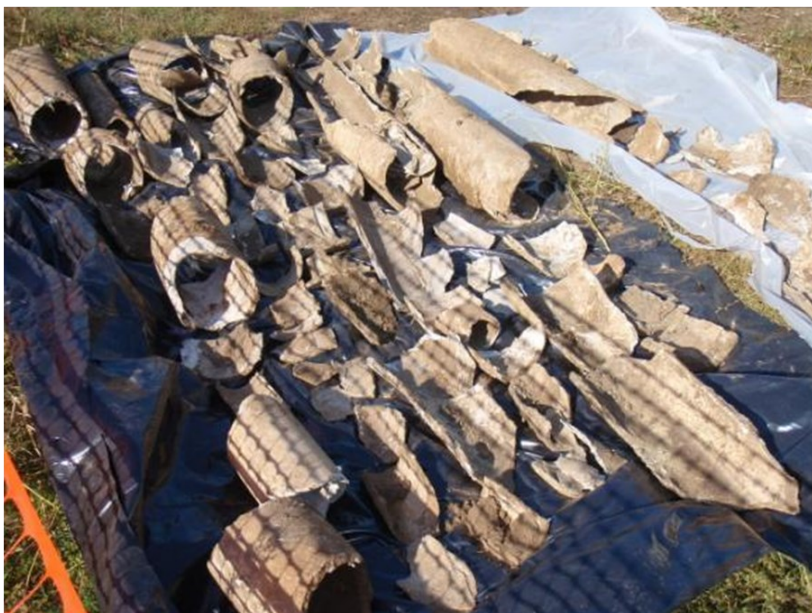
Pieces of the old cement asbestos pipe that was improperly handled by Greiner and Eberhart.
