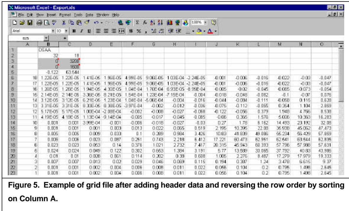
Figure 5. Example of grid file after adding header data and reversing the row order by sorting on Column A.
