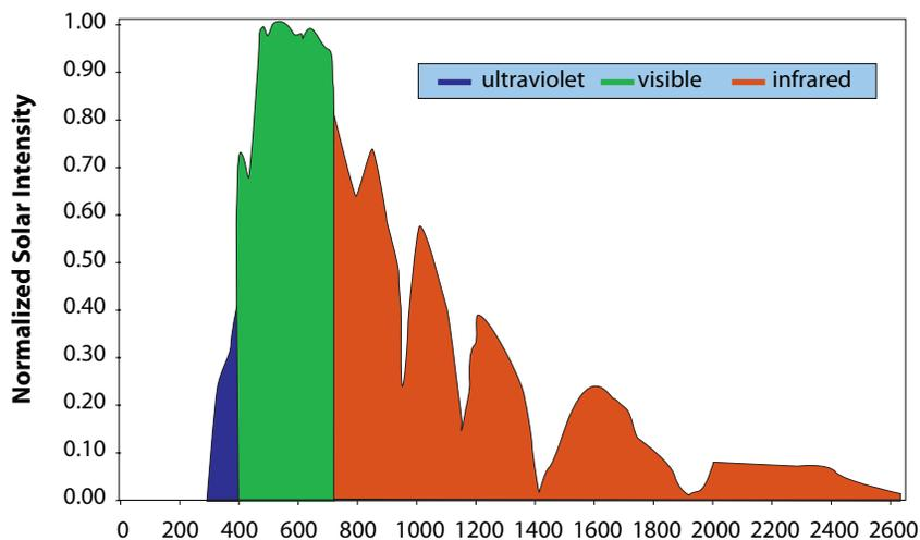
Solar energy intensity varies over wavelengths from about 250 to 2500 nanometers. White or light colored cool roof products reflect visible wavelengths. Colored cool roof products reflect in the infrared energy range.
