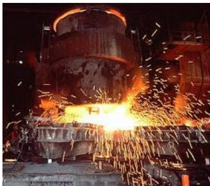
Iron and steel mills are factories where iron ore is reduced, melted, and converted into “pig iron” (an intermediate iron product), finished iron products, or further refined into steel. These facilities may use coke as a fuel to power the furnaces used to melt the iron ore and the forges used to create finished products. Nucor Steel is the only facility in North Birmingham that reported to TRI in the iron and steel mill industry in 2012.<sup>21</sup> For that year,
