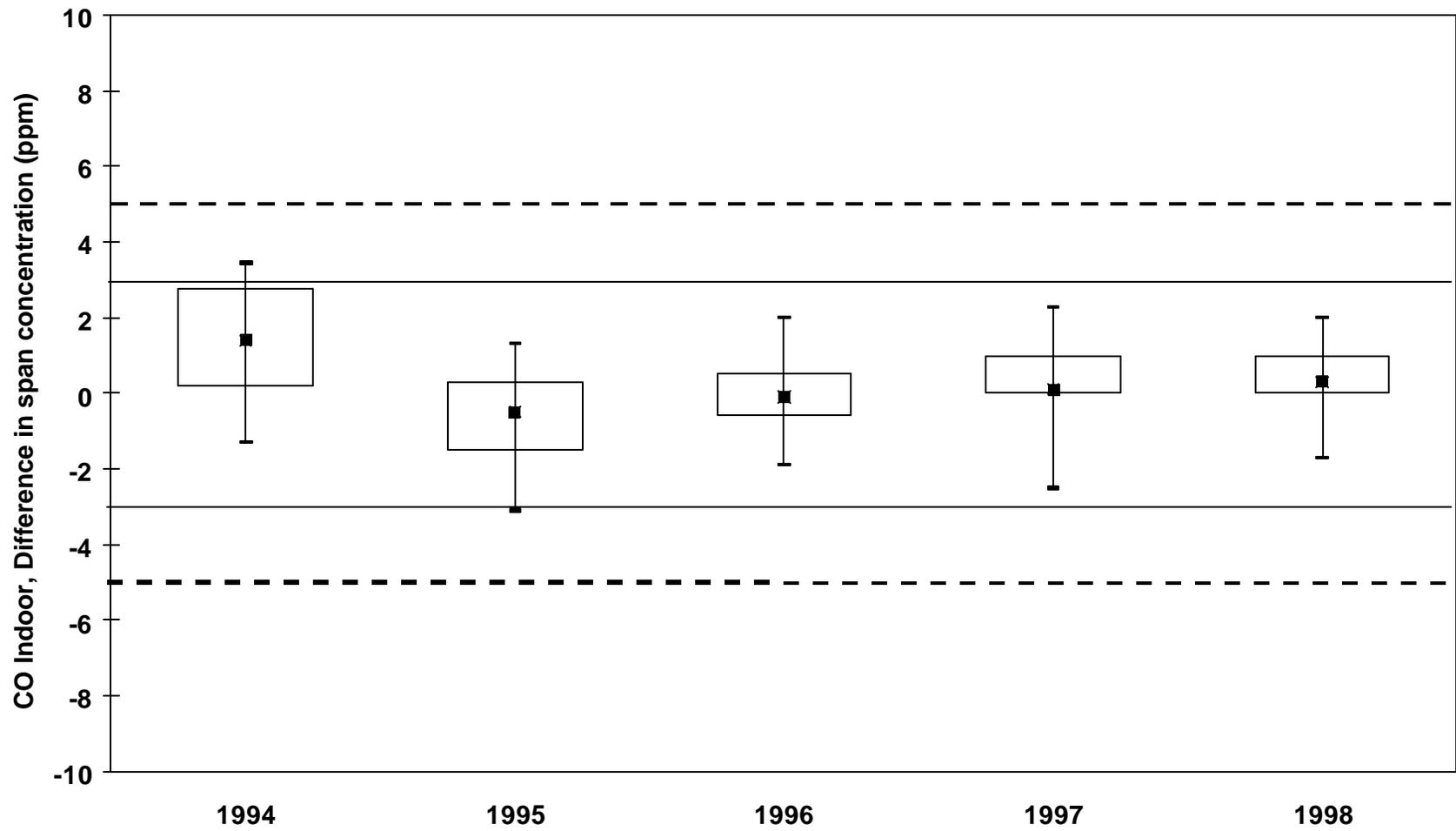
Figure D6 Differential Responses of Indoor CO Sensors to Span Gas
