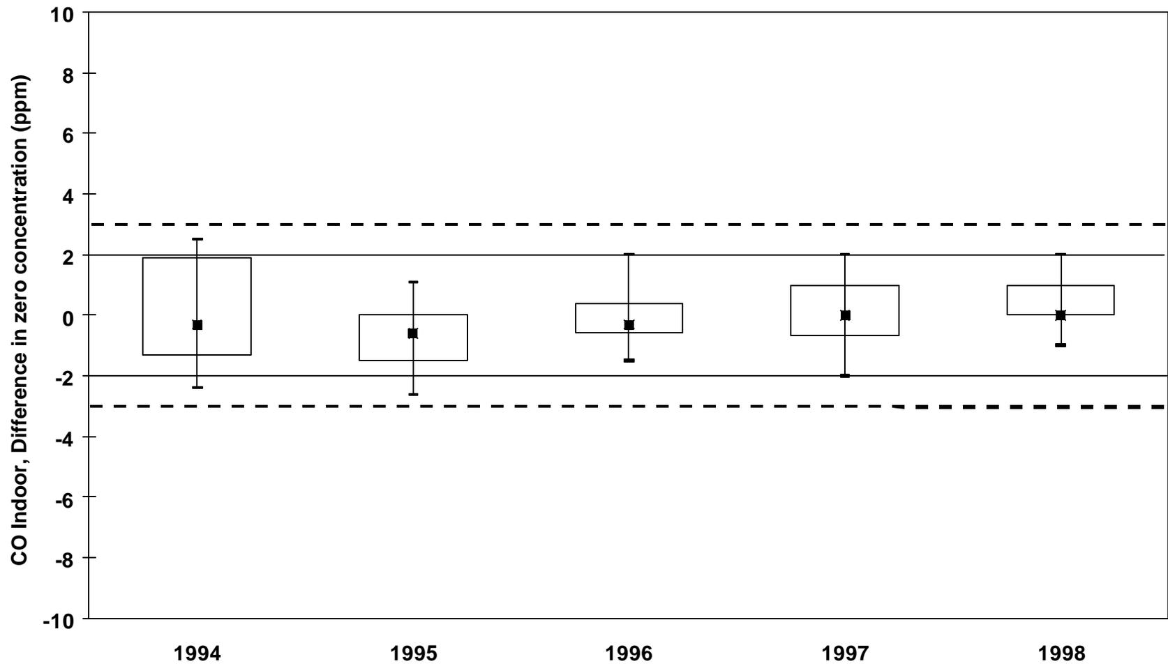
Figure D5 Differential Responses of Indoor CO Sensors to Zero Gas
