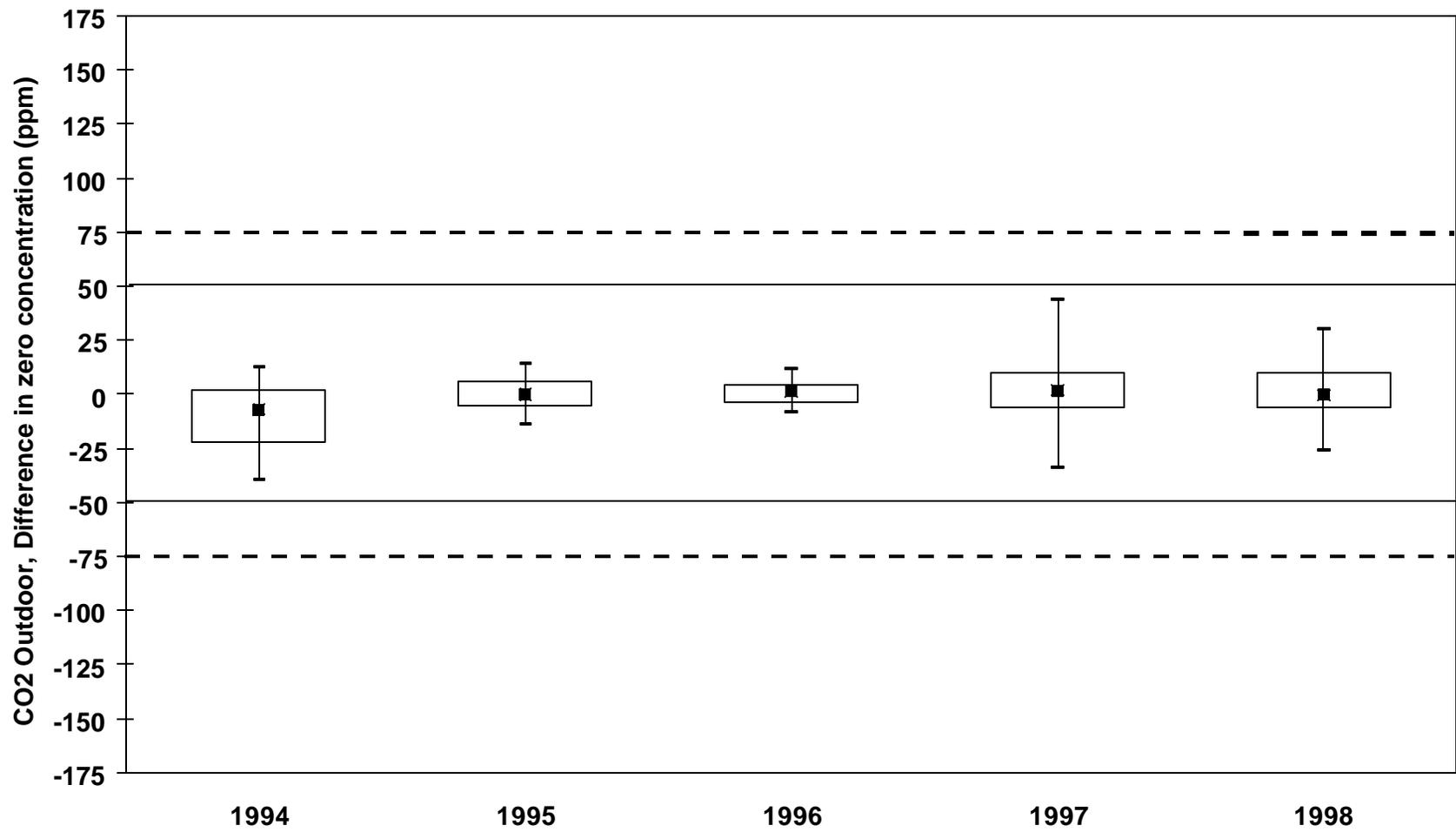
Figure D2 Differential Outdoor CO<sub>2</sub> Sensor Response to Zero Gas, 1994 through 1998
