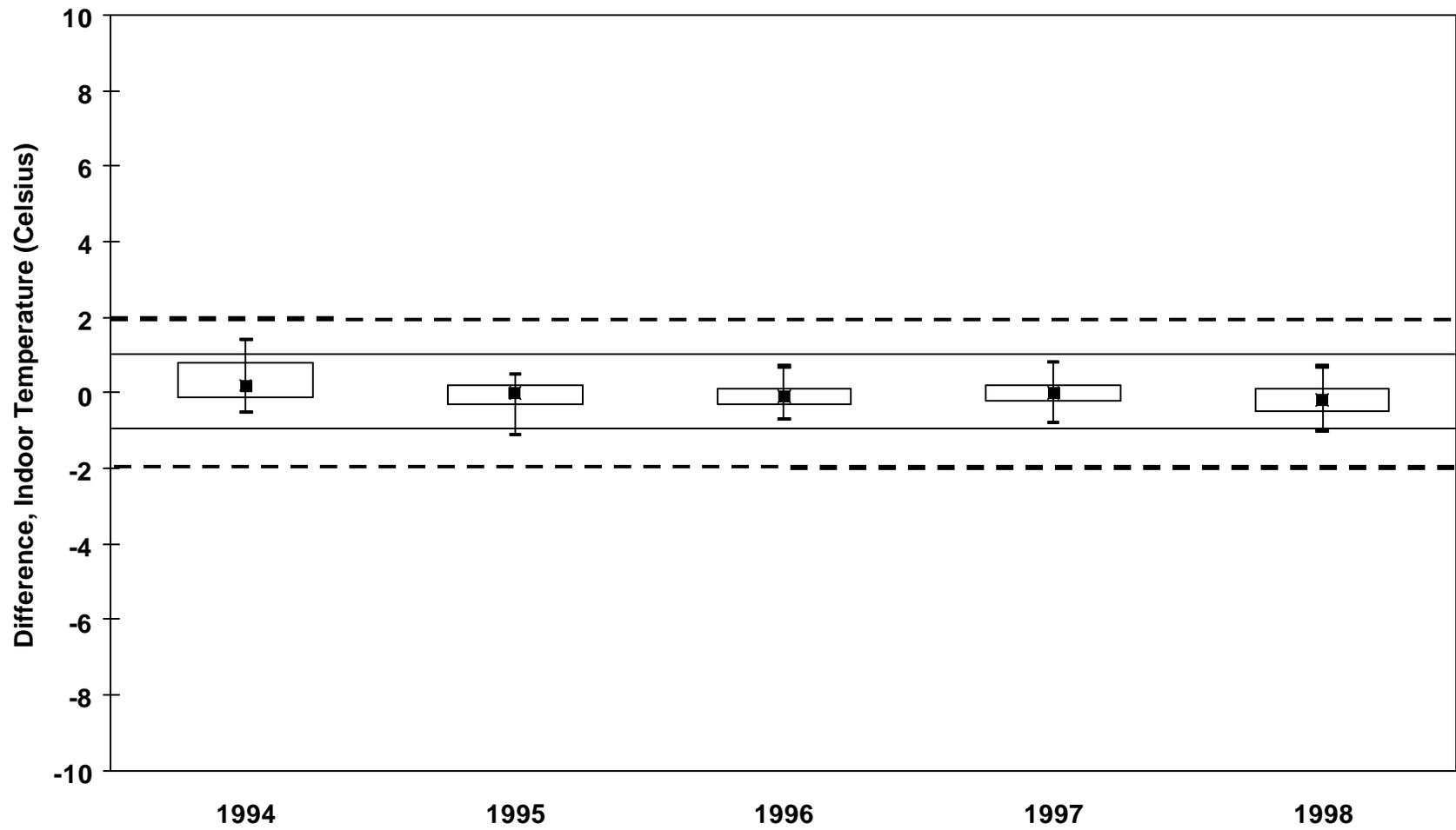
Figure D9 Differential Temperatures from Indoor Sensors Relative to Reference Thermometer
