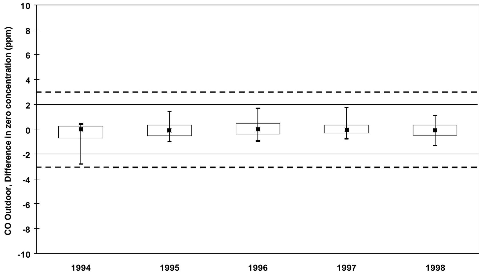
Figure D7 Differential Responses of Outdoor CO Sensors to Zero Gas
