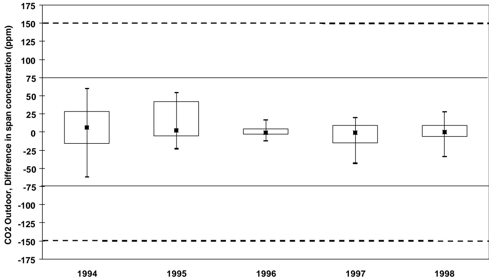
Figure D4 Differential Outdoor CO<sub>2</sub> Sensor Response to Span Gas
