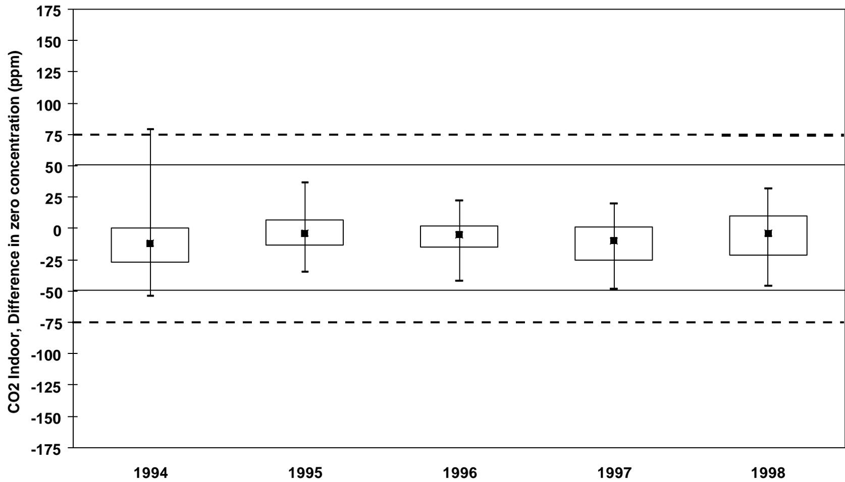
Figure D1 Differential Indoor CO<sub>2</sub> Sensor Response to Zero Gas, 1994 through 1998
