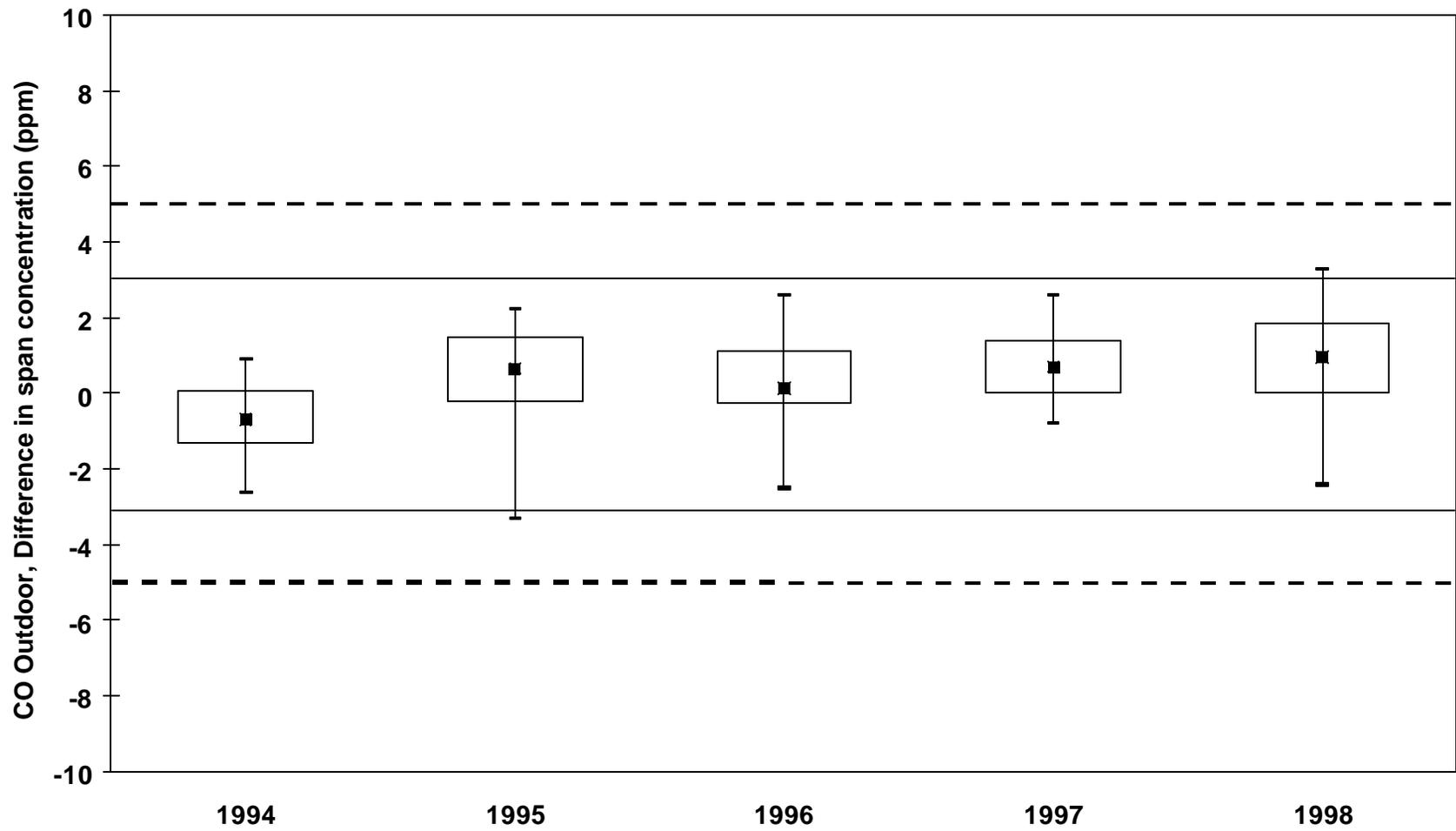
**Figure D8** Differential Responses of Outdoor CO Sensors to Span Gas
