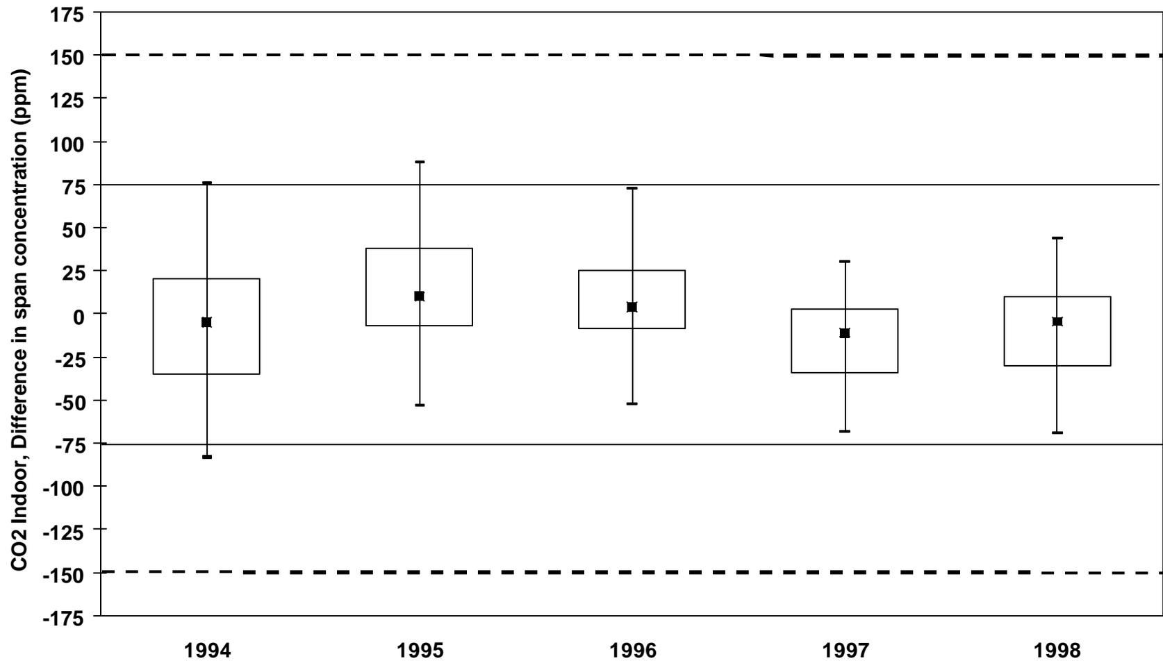
Figure D3 Differential Indoor CO<sub>2</sub> Sensor Response to Span Gas
