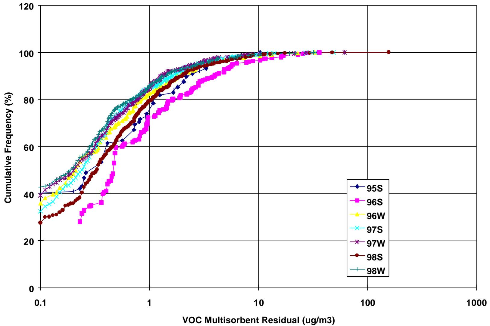
Figure C2 Multisorbent Samplers: Cumulative Frequency of Residuals
