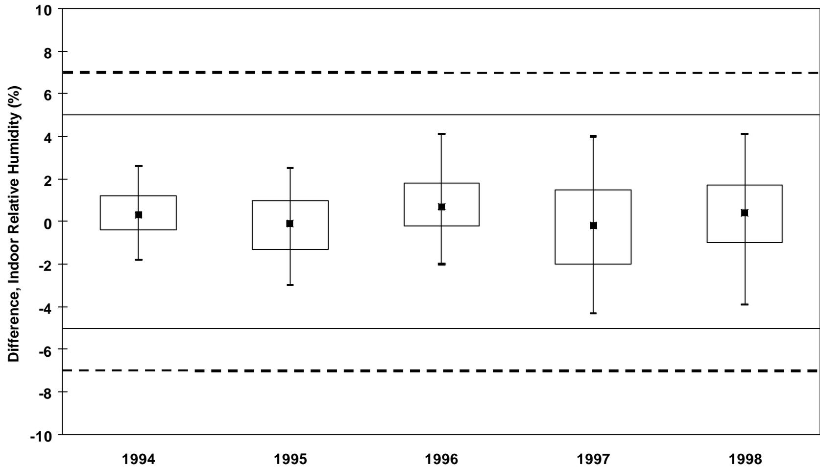
Figure D11 Differential Relative Humidities from Indoor Sensors Compared to Reference Sensor
