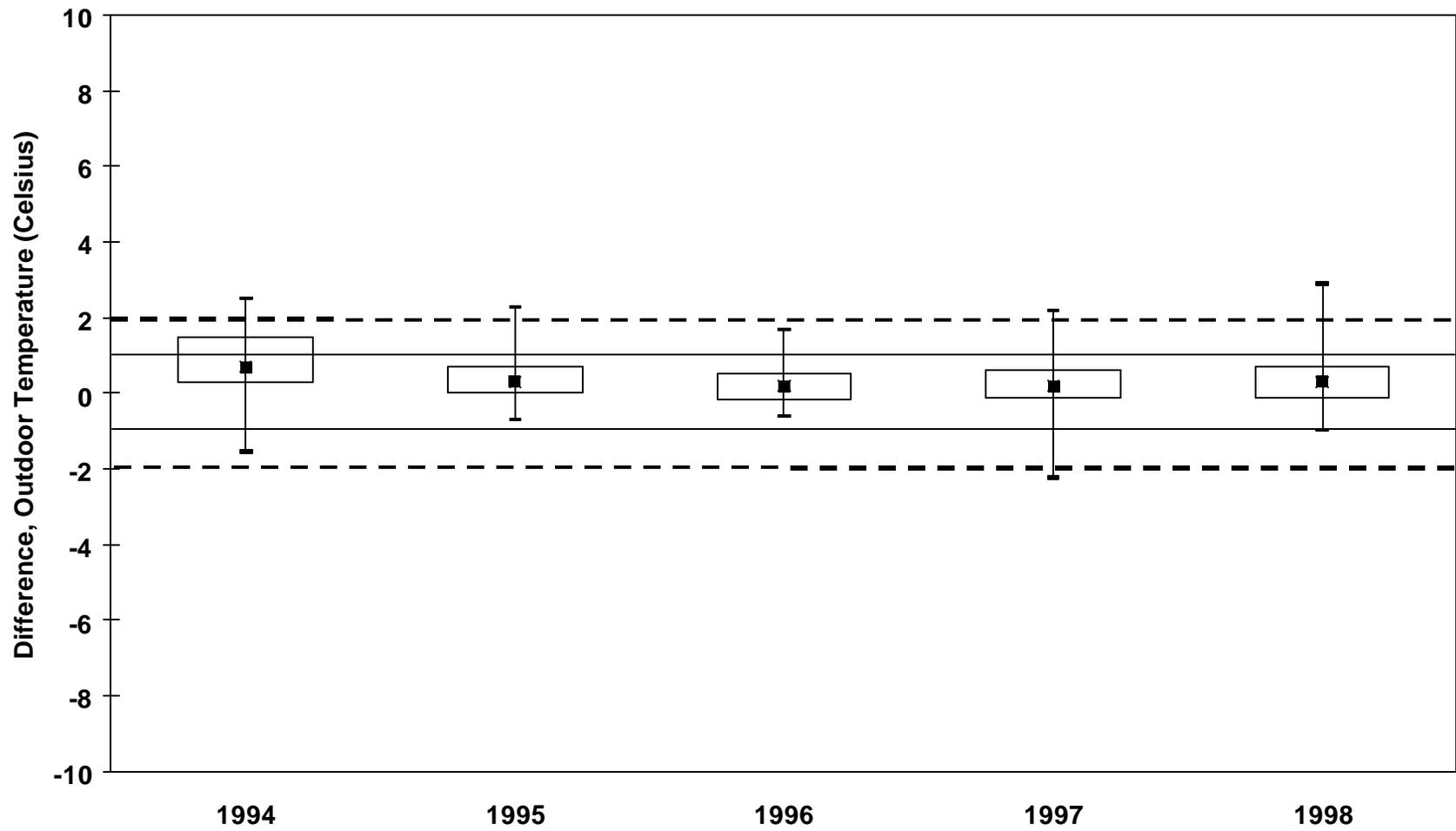
Figure D10 Differential Temperatures from Outdoor Sensors Relative to Reference Thermometer
