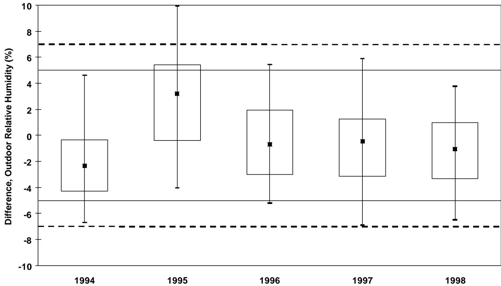
Figure D12 Differential Relative Humidities from Outdoor Sensors Compared to Reference Sensor
