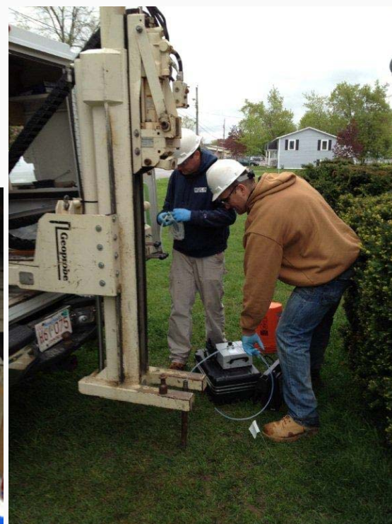
Soil-gas samples via GeoProbe
