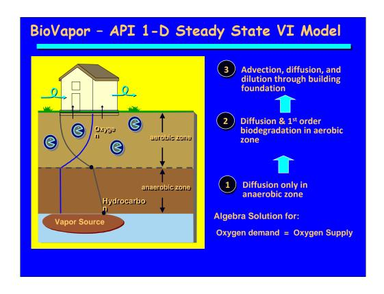
Conceptual model of the API Biovapor model/spreadsheet
