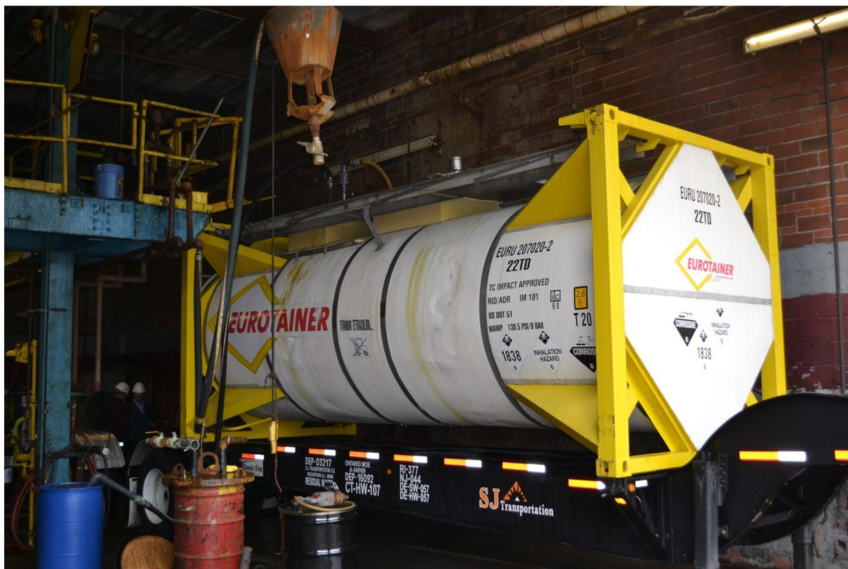
*The tank that Tier employees cleaned out which caused the release of hydrochloric gas.*
