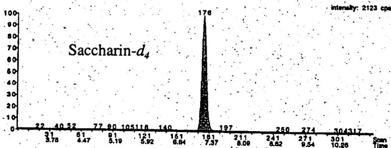
Figure 4 contd. Representative ion chromatograms from the analysis of Washington soil fortified at 1 ppb with MKH 6561 carboxylic acid, MKH 6561 sulfonamide acid, saccharin and 4-hydroxy saccharin.
