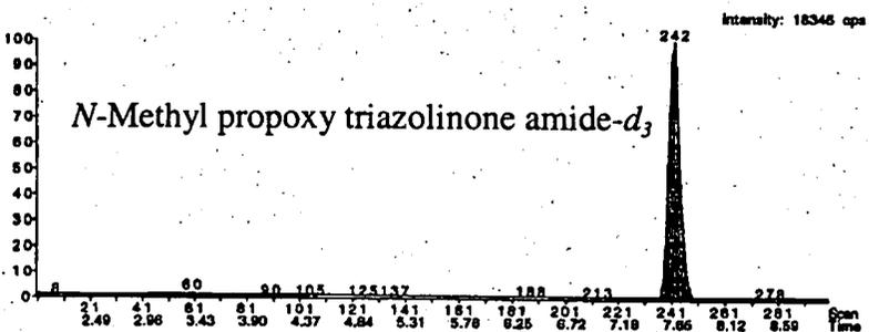
Figure 1 contd. Representative ion chromatograms from the analysis of unfortified Washington soil (control) for MKH 6561, *N*-methyl propoxy triazolinone, *N*-methyl propoxy triazolinone amide and MKH 6561 sulfonamide methyl ester.
