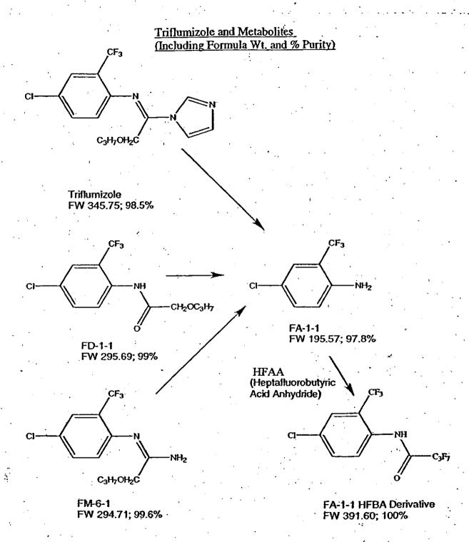
Figure 2. Scheme Showing Conversion of Triflumizole and Degradates to FA-1-1 and Conversion of FA-1-1 to the HFBA Derivative.
