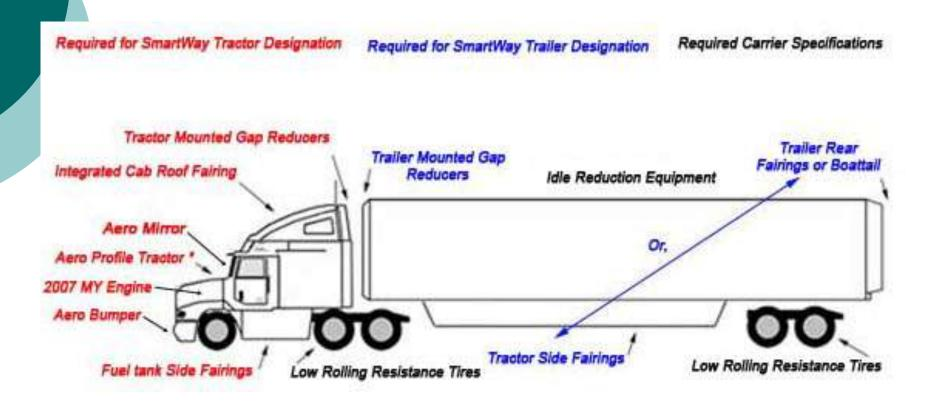
2007 engine and fuel savings of 10% to 20% compared with truck without these features
