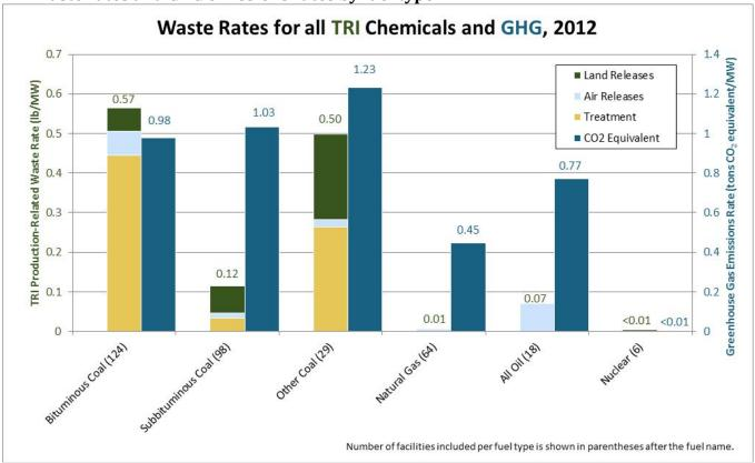
This figure shows TRI waste management rates and GHG emission rates for facilities in the electric utilities industry that reported to both TRI and the GHGRP for 2012, the most recent year for which the facility-level fuel use data are available. By fuel type, the figure shows:
