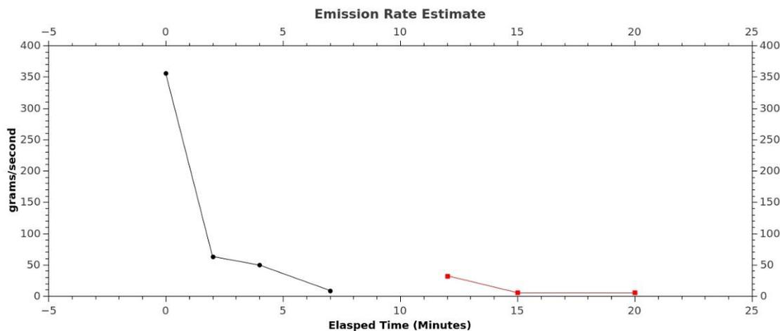
Figure 9. ASPECT Developed Ammonia Emission Rates
