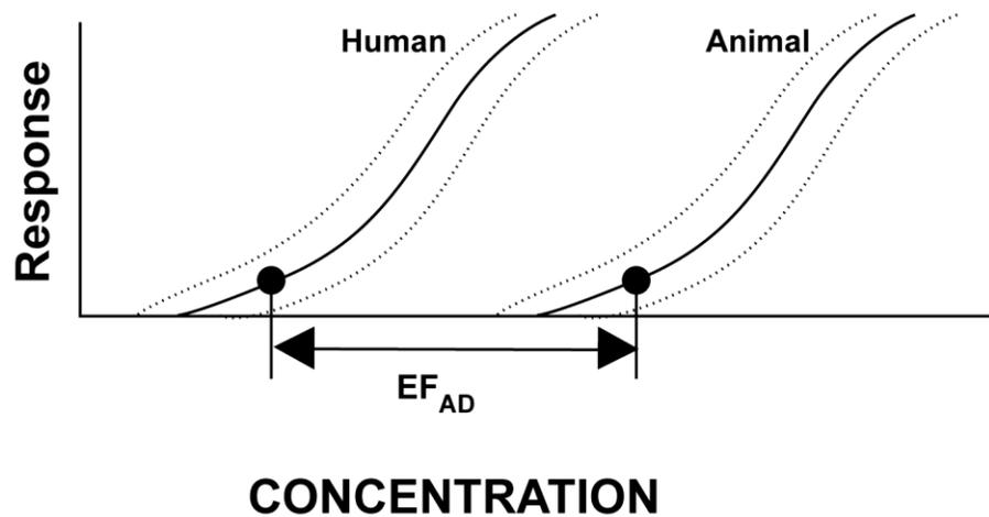
**Figure 6. Interspecies toxicodynamics.** The TD difference between test animals and humans is calculated from concentration-response relationships determined in test systems or animals generally representative of the respective species. The comparison is made for concentrations producing the same level of response, and comparisons are made using values representing the central tendency. Dashed lines represent variability.
