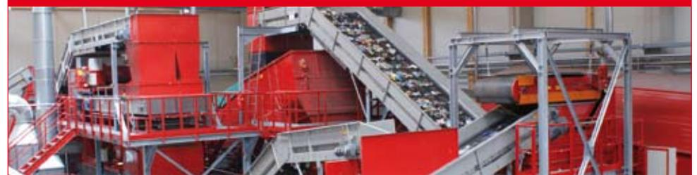
ONE OF THE TYPICAL SORTING TASKS WHICH ARE BUILT-IN IN OUR PLANT ARE SORTING OF POLYMERS ACCORDING TO THEIR TYPE OF MATERIAL (PET, HDPE, PP, PS, MIXED POLYMERS, ETC) AND BEVERAGE CARTONS.
