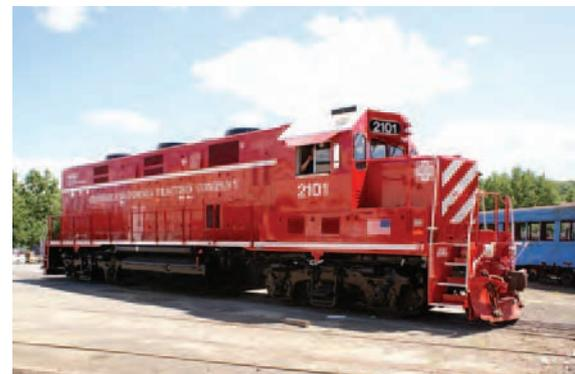
This new diesel-electric hybrid locomotive, purchased with partial funding from EPA, is cleaner and uses 50% less fuel than its predecessor on a freight line in California's San Joaquin Valley. Far right: Improved air quality in Los Angeles.
