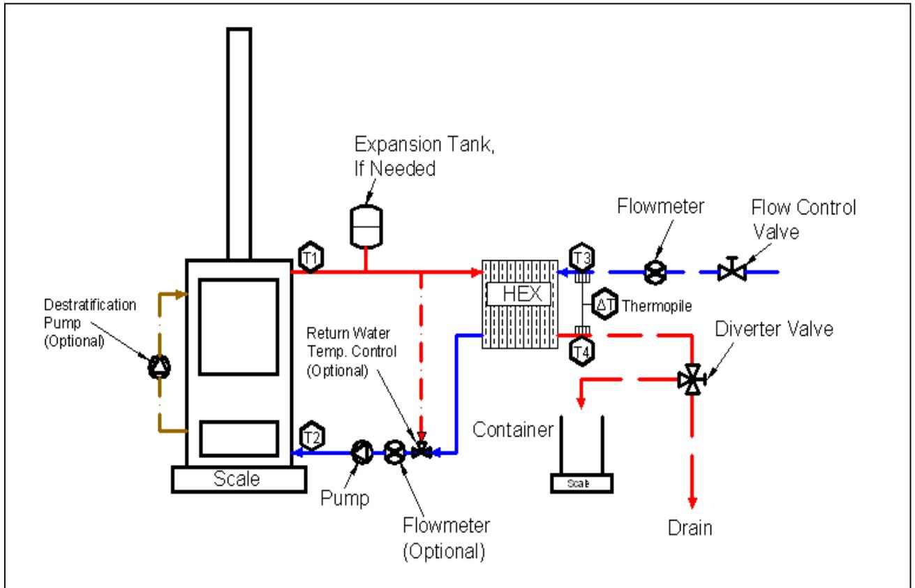
**Note:** Illustrated appliance pump location and flow path through the appliance.
