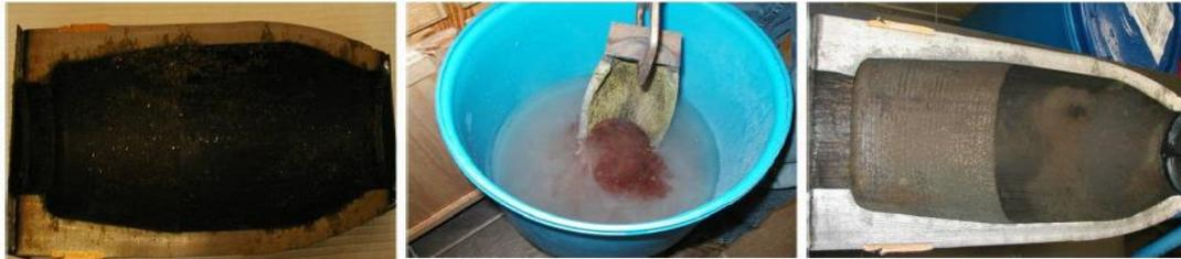
Rapid decontamination of halved bomb casings before
