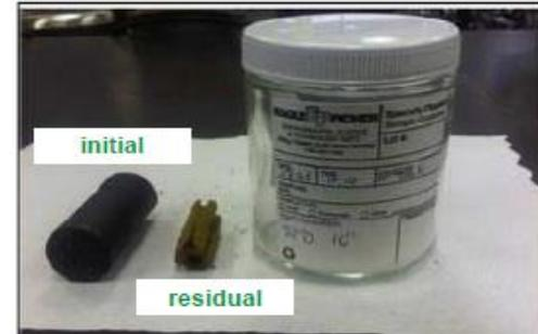
33g of NC propellant reduced to <5g of non-explosive residual in less than 48 hours
