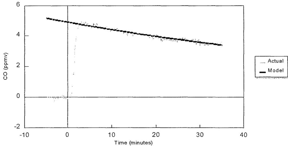
Figure 4.4. Concentration of a Target Inorganic Gas (CO) Versus Time.
