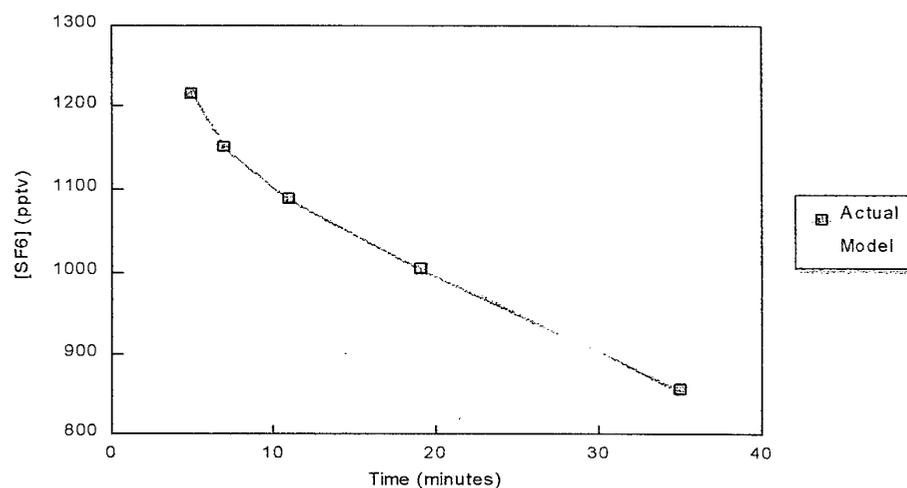
Figure 4.1. Concentration of SF<sub>6</sub> Tracer Gas Versus Time.
