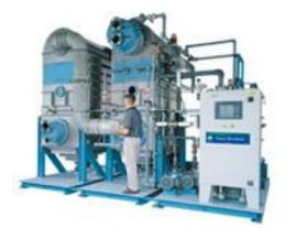
Typical Heavy Waste Water concentration systems: Step One (Samsco & Metsco company references) System capacities range from 300 to 4000 gals/day : about 60% water reduction maximum
