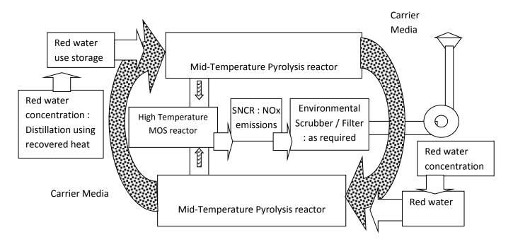
Specific treatment of the gas and solids by-products of this processing technology is considered integral to the success of any installation. Combined reuse of energy flows and balances are also considered, many times uniquely, due to considerations concerning feed stocks, effluents, and process/equipment cost/design.
