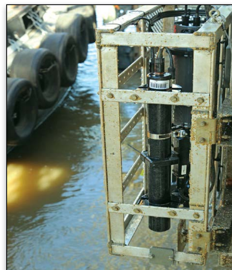
Continuous ultraviolet nitrate sensors and other water quality instruments deployed in the Mississippi River allow for a better understanding of nitrogen dynamics at the rates in which changes occur.
