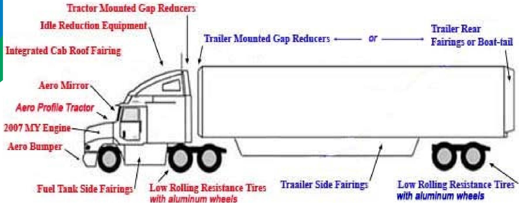
Potential fuel savings – 10% - 20% (on-highway operation) compared to a truck without these features
