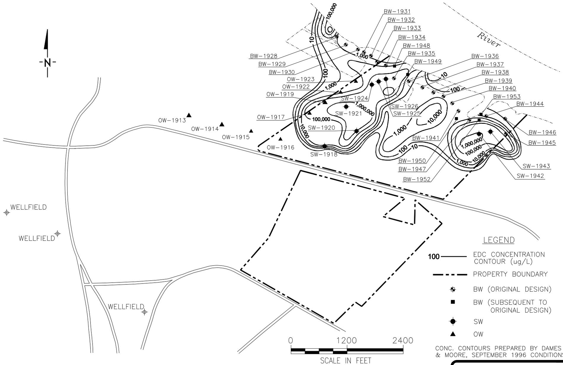
Figure 4-3. EDC concentrations and current remediation wells, Kentucky.
