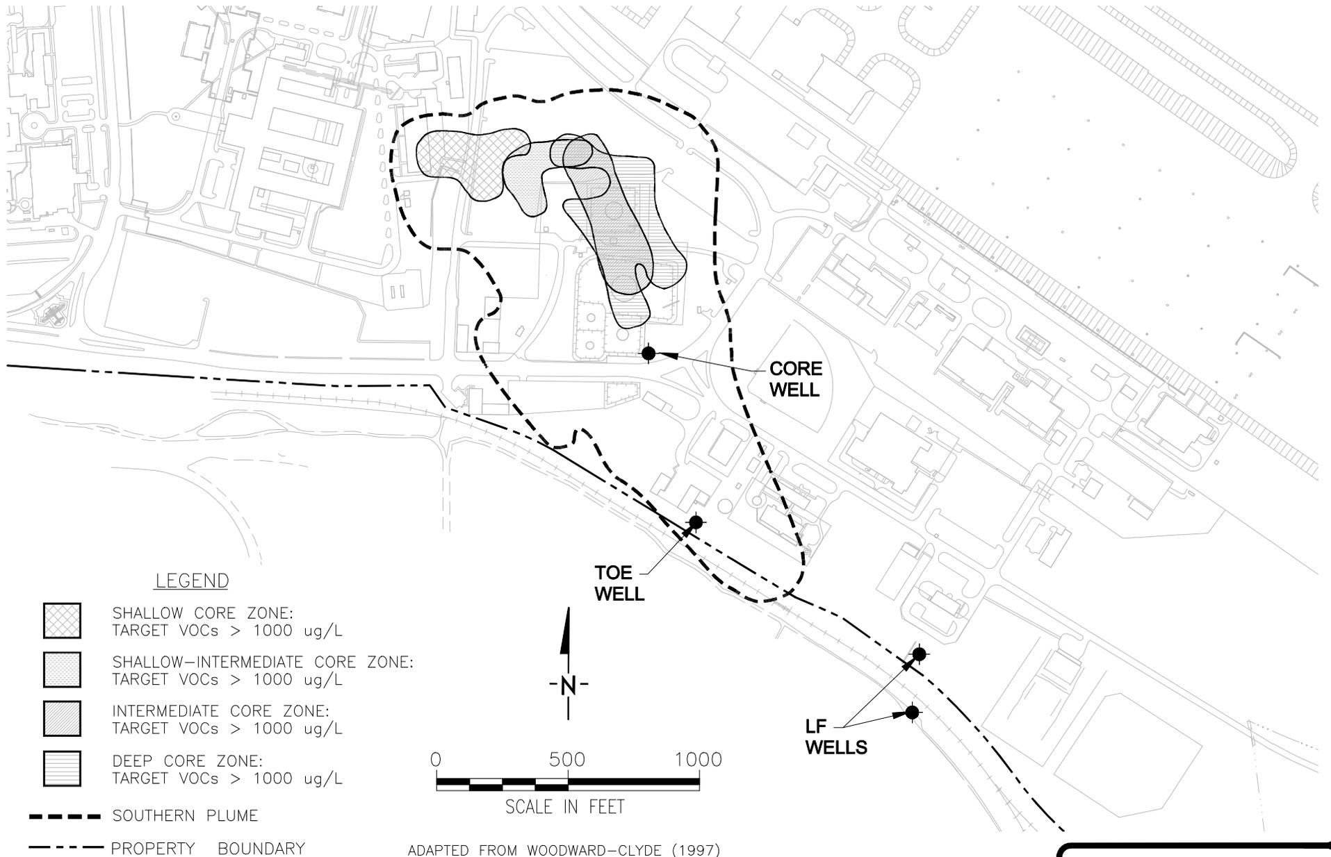
Figure 6-3. Southern plume and current remediation wells, Offutt.
