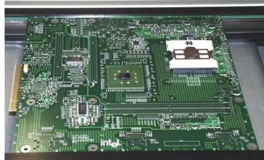
**Figure 2. Reflow test PWB assembly**
