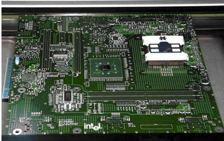
**Figure 2-13. Reflow Test PWB Assembly**
