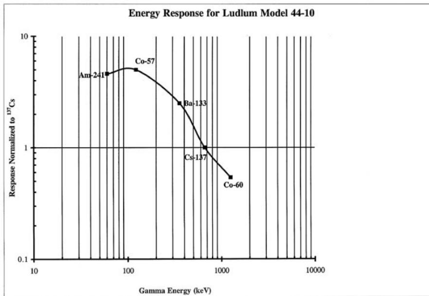
**FIGURE 2 – Gamma Energy Response for a Na(Tl) detector**
