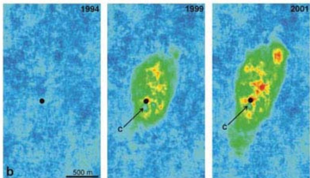
The CO<sub>2</sub> created impedance contrasts that revealed thin shale baffles within the reservoir.
