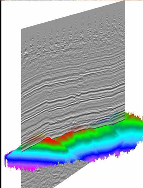
For all relevant cases, this involves an impermeable unit above the injection zone. This mechanism is effective unless the physical barrier is breached (e.g., faults, wells)
