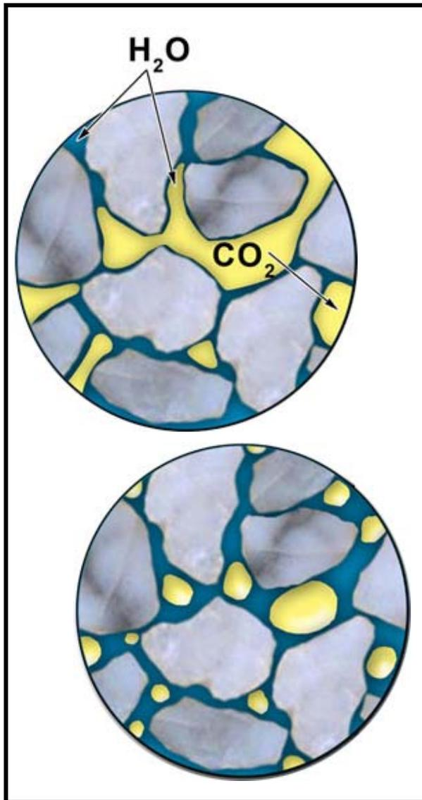
At high pore saturations, CO<sub>2</sub> is mobile and can move as a supercritical phase. At low saturations, CO<sub>2</sub> is trapped by the capillary forces, and will only move by intervention.
