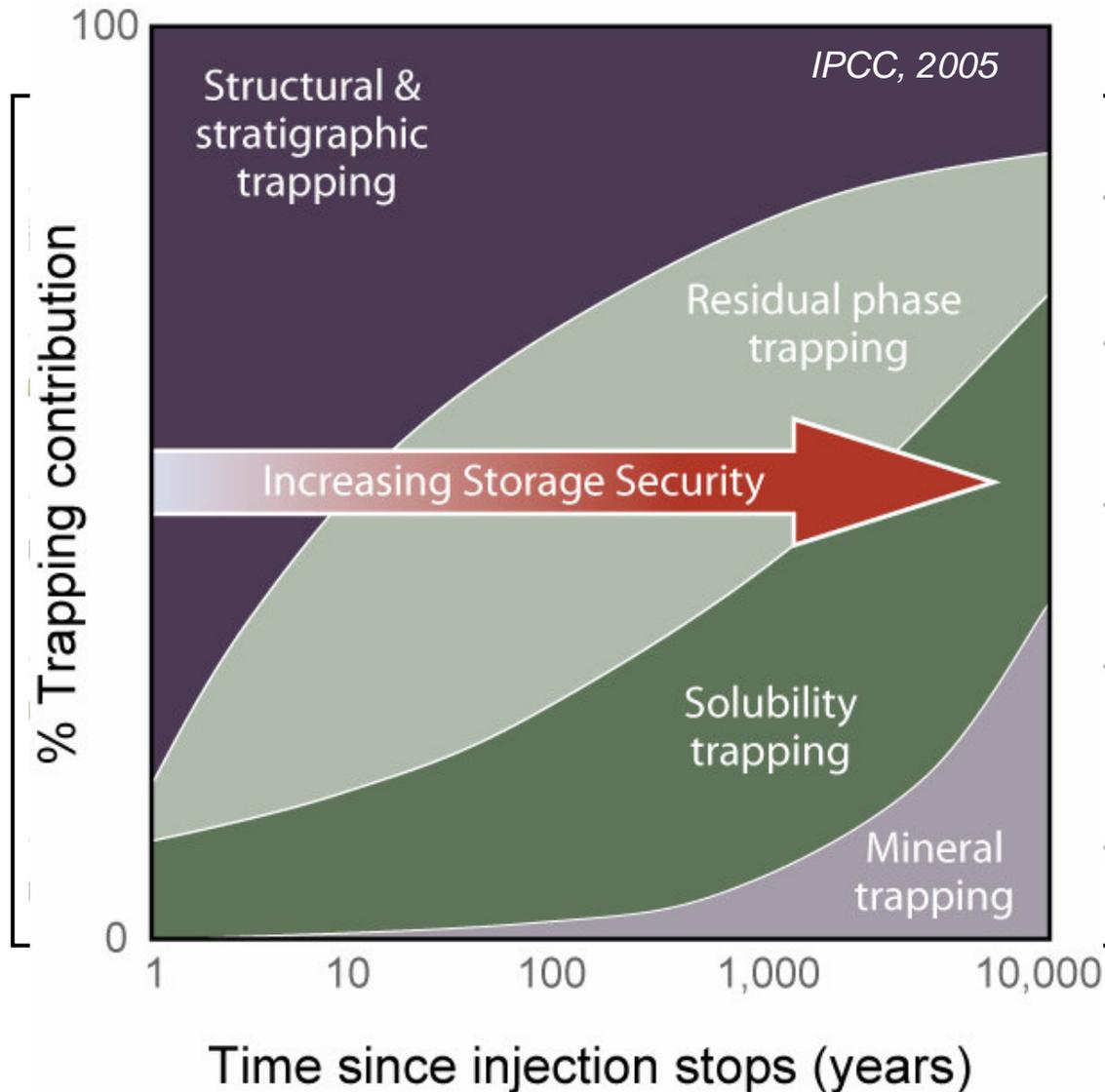
**Because of multiple storage mechanisms working at multiple length and time scale, the shallow crust should attenuate mobile free-phase CO<sub>2</sub> plumes, trap them residually, & ultimately dissolve them**
