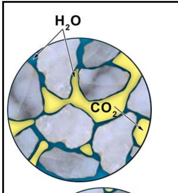
At high pore saturations,  $CO_2$  is mobile and can move as a supercritical phase. At low saturations,  $CO_2$  is trapped by the capillary forces, and will only move by intervention.
