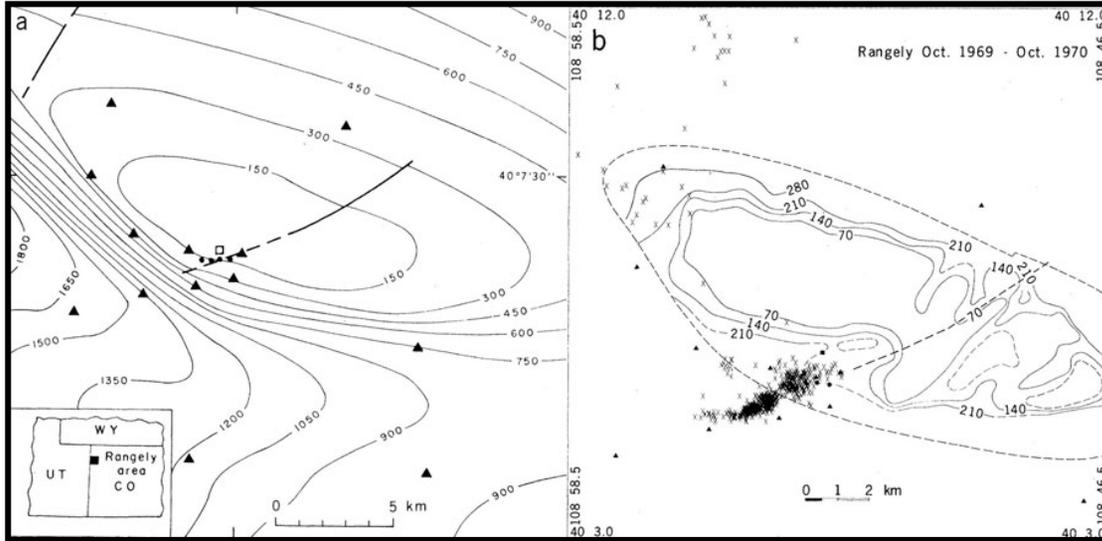
An experiment at Rangely field, CO, attempted to induce earthquakes in 1969-1970. It did so, but only after enormous volumes injected over long times on a weak fault
