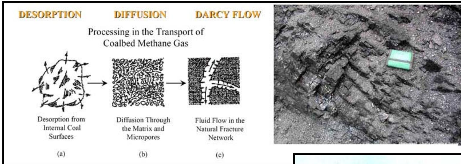
Coal storage (and ECBM) are fundamentally different. Here,  $\text{CO}_2$  adsorbs to the organic mineral surface. In doing so, it may liberate  $\text{CH}_4$  at  $\sim 2:1$ . The  $\text{CO}_2$  is not mobile and does not need to be supercritical.
