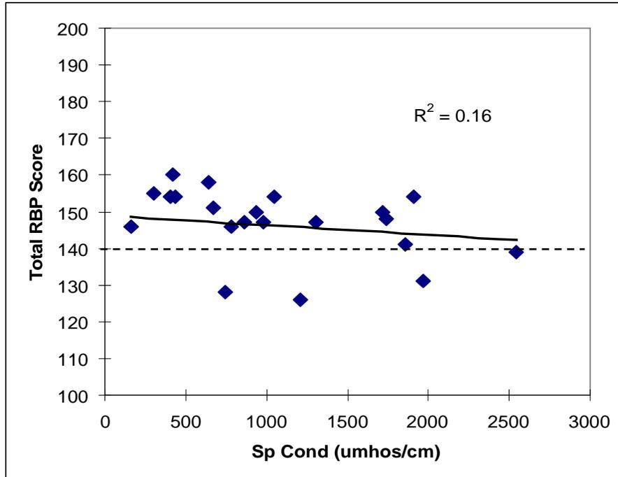
**Figure A2.5. Relationship between RBP habitat score and specific conductance obtained from receiving streams of mine site impoundments, indicating a poor correlation. Data from Pond et al. (2008). Dashed line demarcates criterion required for WVDEP reference site candidacy.**
