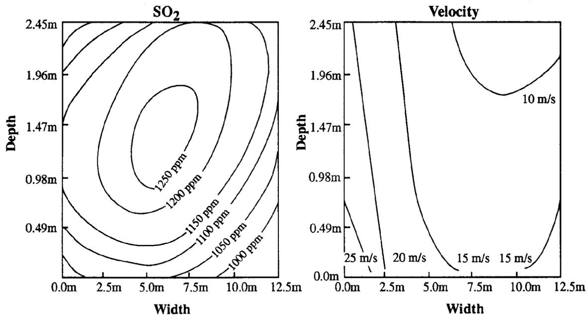
**Figure 2-2. Stratification in Gas Concentration and Flue Gas Velocity (Gregory et al., 1976)**
