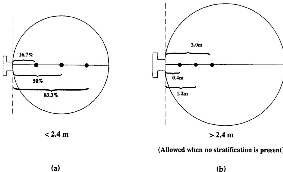
**Figure 2-3. Gas Sampling Reference Method Traverse Points Specified in 40 CFR 60 Appendix B**
