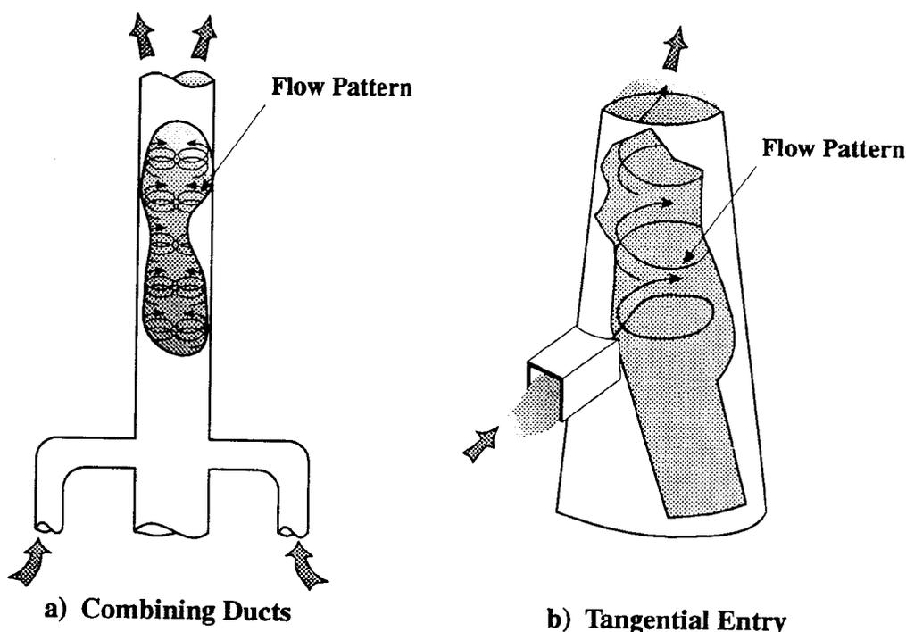
**Figure 2-5. Conditions Under Which Flow Stratification or Cyclonic Flow Conditions May Occur**
