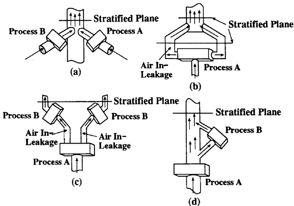
**Figure 2-4. Conditions Under Which Gas Concentration Stratification May Occur (after Zakak et al., 1974)**
