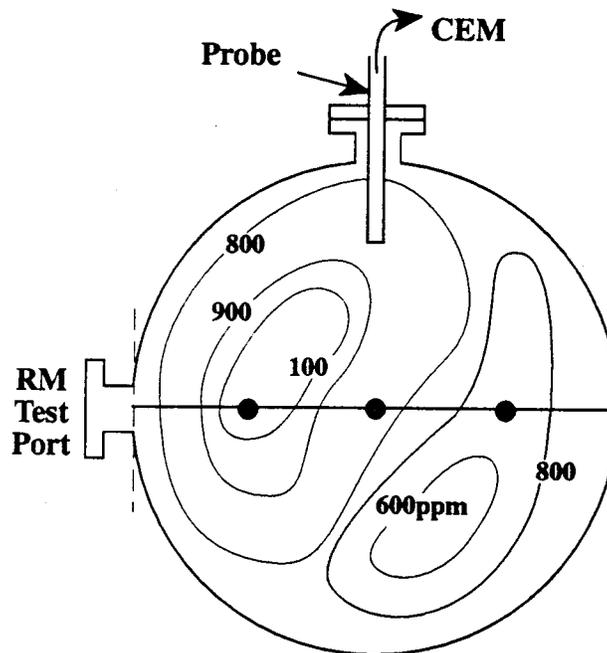
**Figure 2-1. Stratification and Reference Method Testing in a Stack**
