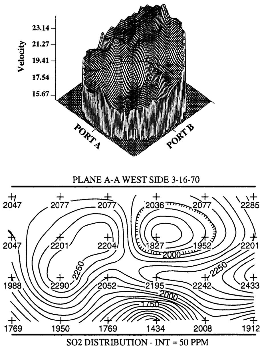
Figure 2-6. Velocity and Gas Concentration Profiles
